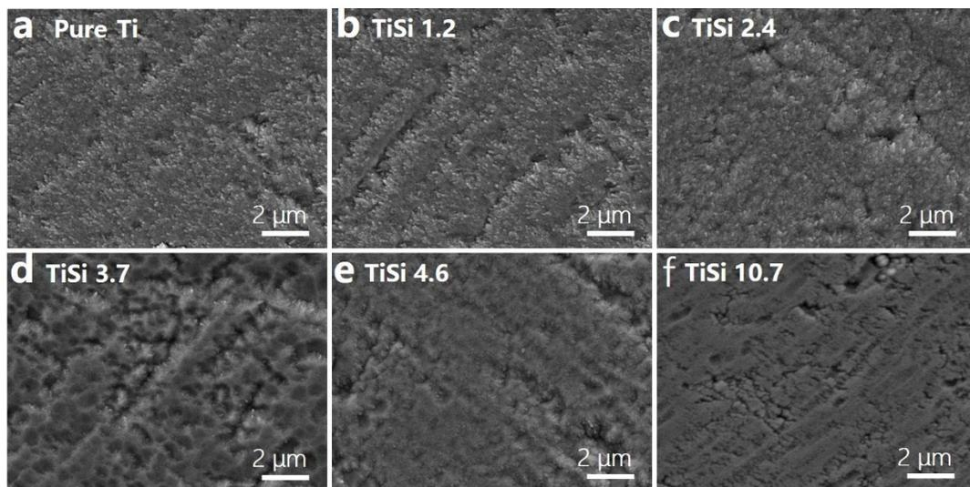
**Fig. S1** SEM images of pure Ti coating (a) and TiSi coatings with different Si contents: (b) 1.2at%, (c) 2.4at%, (d) 3.7at%, (e) 4.6at% and (f) 10.7at%.
