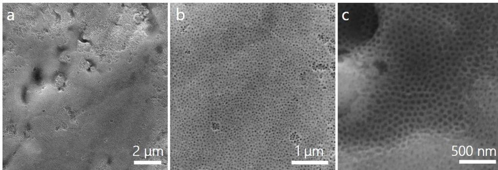
**Fig. S5** Surface morphologies of different magnification of the anodized samples from the TiSi coating of 10.7wt.% Si content.
