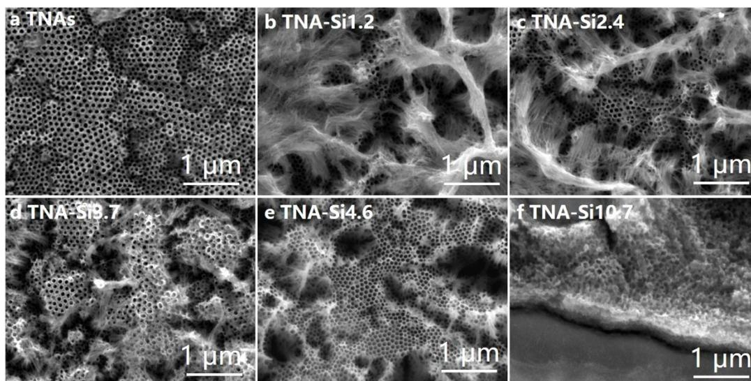
**Fig. S3** Surface morphologies of TNAs (a) and TNA-Sis (b-f) anodized in ethylene glycol electrolyte supplemented with 0.3 wt%  $\text{NH}_4\text{F}$  and 2.0 vol%  $\text{H}_2\text{O}$  at 30 V and room temperature for 4 h.
