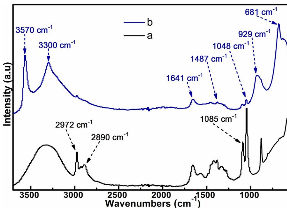
**Figure S3** FTIR spectra of (a) initial solid nanoparticles (black line) and (b) hollow multipod Cu(OH)<sub>2</sub> superstructure (blue line).
