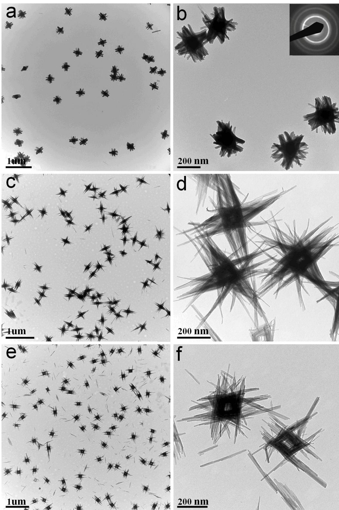
**Figure S1** Characterization of irregular  $\text{Cu}(\text{OH})_2$  nanoparticles: (a) low-magnification and (b) high-magnification TEM images (inset is SAED). The samples prepared from the synthesis for TEM with reacted different concentration of  $\text{NH}_3$ : c) and d) 400  $\mu\text{L}$ ; e) and f) 800  $\mu\text{L}$ .
