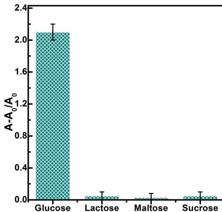
**Figure S6** Selectivity analysis for glucose detection by monitoring relative absorbance in buffer (pH was 4.5 and temperature was 25 °C). Glucose concentration = 0.1 mM, and the other sugars are 5 mM.
