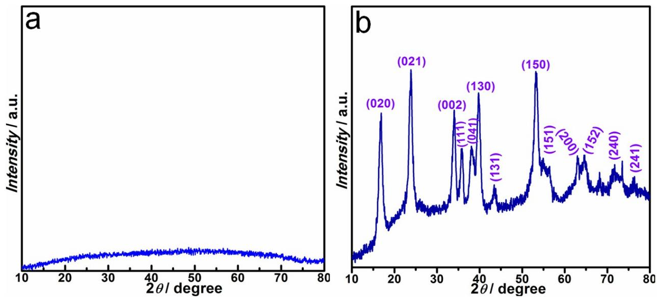
**Figure S2.** XRD patterns of a)  $\text{Cu}(\text{OH})_2$  nanoparticles and b) the samples prepared from the synthesis for TEM with reacted  $800 \mu\text{L NH}_3$  (Figure S1 c-d);.
