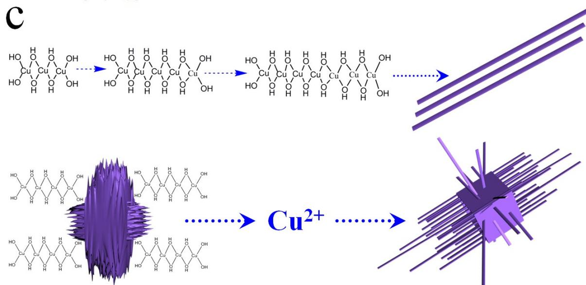
**Figure S4** Schematic of (a)  $[\text{Cu}(\text{H}_2\text{O})_6]^{2+}$  coordinating with  $\text{NH}_3 \cdot \text{H}_2\text{O}$  to generate  $[\text{Cu}(\text{NH}_3)_n]^{2+}$ ; (b) coordinated growth of the lamellar structure; (c) formation of tiny branch and hollow multipod  $\text{Cu}(\text{OH})_2$  superstructure.
