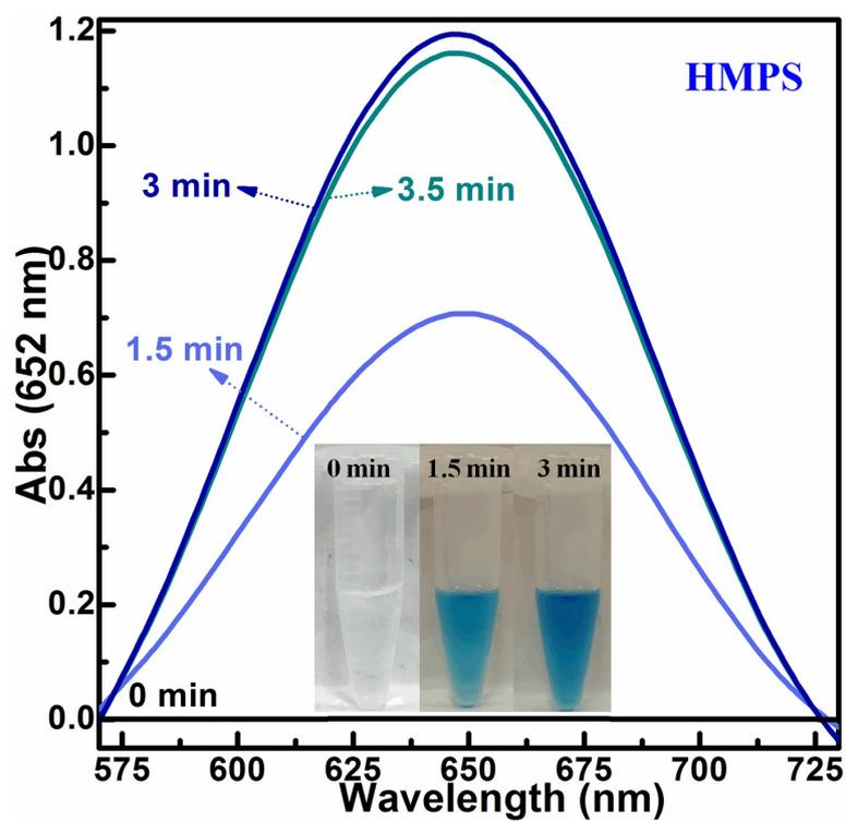
**Figure S5** The absorption spectra for TMB oxidation by HMPS in the presence of  $\text{H}_2\text{O}_2$  to produce blue ox-TMB (pH was 4.5 and temperature was 25 °C); the above inset corresponds to typical photographs of the reaction solution.
