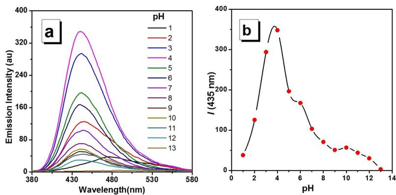
**Figure S4.** (a) Emission spectra of TPE-CA (10  $\mu$ M) in THF/ buffer solution (volume fractions of buffer solution is 99%) with different pH values. (b) Plot emission intensity ( $I$ ) at 435 nm in different pH.
