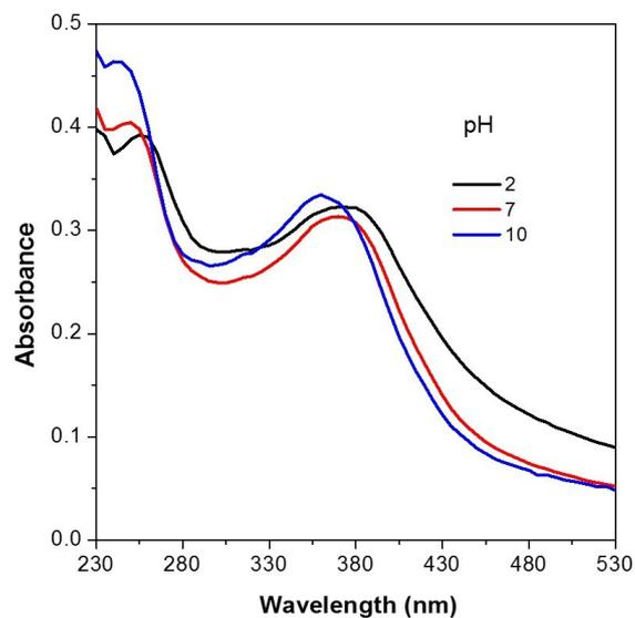
**Figure S5.** Effect of different pH on the absorption spectra of TPE-CA in THF/buffer solution (3: 7, v/v). The concentration of TPE-CA was 10  $\mu\text{M}$ .
