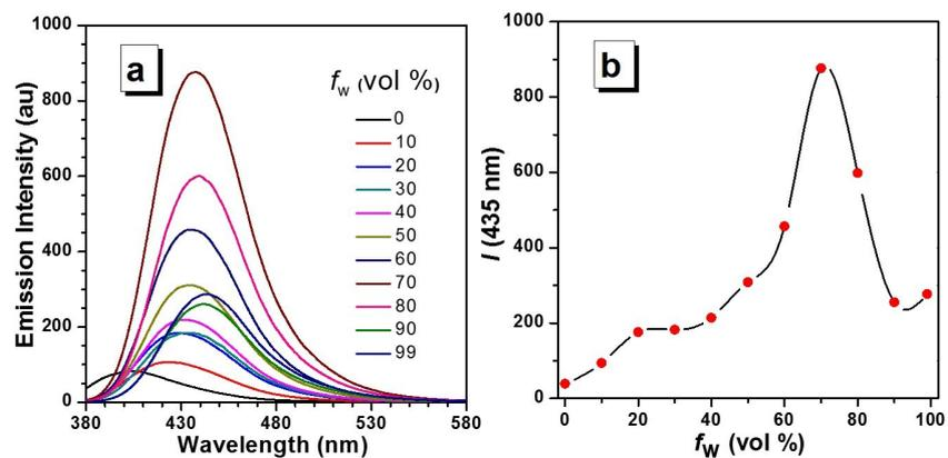
**Figure S3.** (a) Emission spectra of TPE-CA (10  $\mu$ M) in THF/buffer solution (HEPES, PH=7.4) mixtures with different volume fractions of buffer solution ( $f_w$ ). (b) Plot emission intensity ( $I$ ) at 435 nm versus buffer solution fraction.
