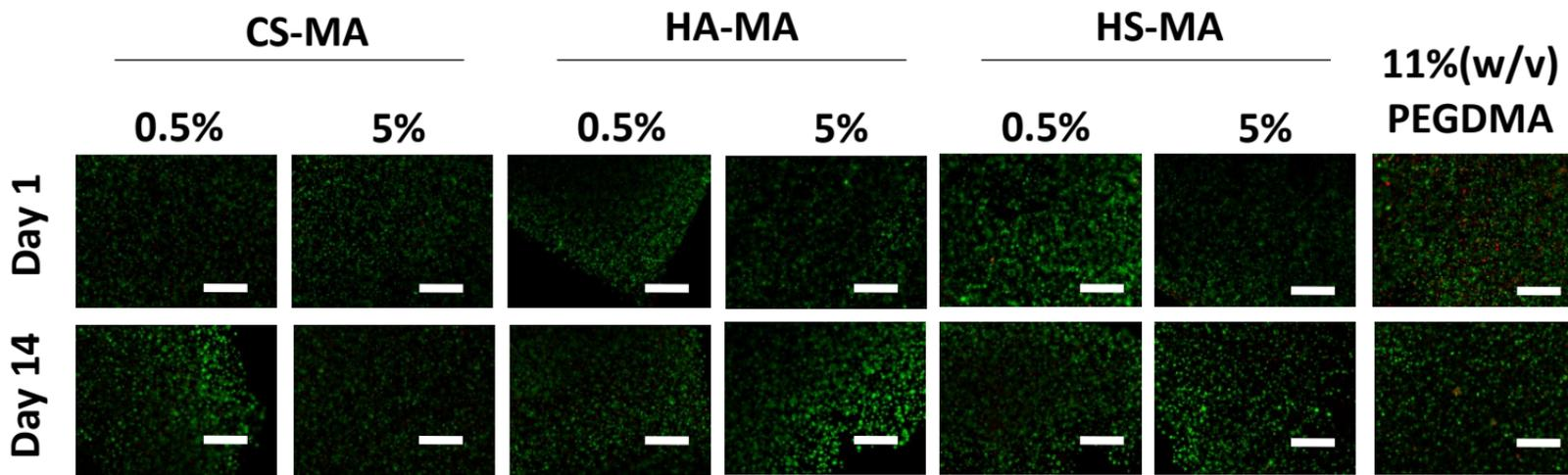
Figure S1: Neonatal chondrocyte (NChon) viability assayed via the LIVE/DEAD kit on day 1 and day 14 after encapsulation in 11% PEGDMA hydrogels. ECM molecules were added to the hydrogels as indicated. Scale bar, 400  $\mu\text{m}$ .
