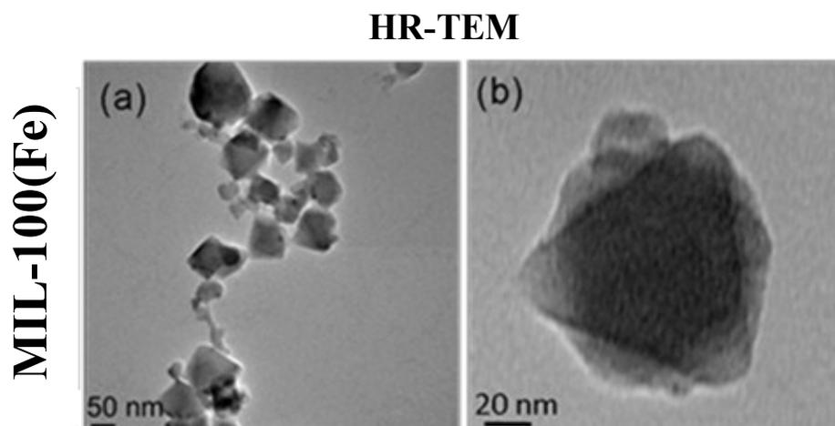
**Figure S1.** HR-TEM images of MIL-100(Fe) NPs. The scale bar corresponds to (a) 20  $\mu\text{m}$  and (b) 50  $\mu\text{m}$ .
