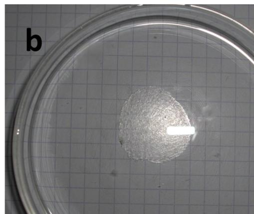
**Figure S10.** Press molded PVA wafer after different times. a) two days; b) one week
