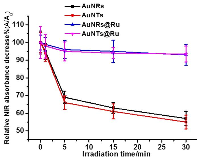
**Figure S8.** The photothermal stability of AuNRs@Ru and AuNTs@Ru in comparison with AuNRs and AuNTs; extinction peak shifts as a function of irradiation time (0-30 min, 0.25 W/cm<sup>2</sup>) were recorded.
