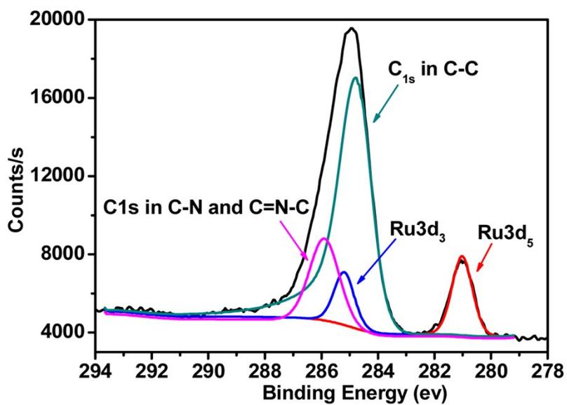
**Figure S2.** Energy distributions of the elements Ru<sub>3d</sub> and C<sub>1s</sub> in the AuNRs@Ru as determined by XPS measurements.
