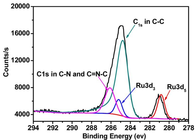
**Figure S3.** Energy distributions of the elements Ru<sub>3d</sub> and C<sub>1s</sub> in the AuNTs@Ru as determined by XPS measurements.
