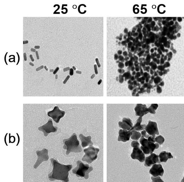
**Figure S9.** The stability of AuNRs (a) and AuNTs (b) at 25 °C and 65 °C incubation for 30 min, respectively.
