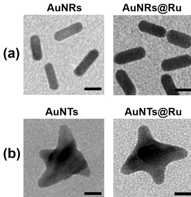
**Figure S1.** The high resolution TEM (HR-TEM) images of the (a) AuNRs and (b) AuNTs before and after modification with the Ru complex.
