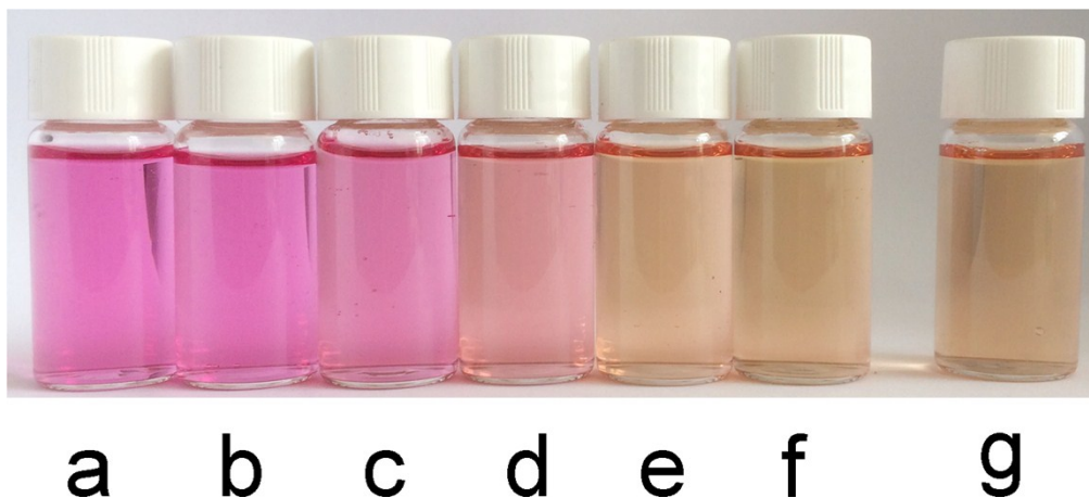
Fig. S6 Color photographs of xylenol orange solution at pH 7.4 in the presence of 20 \mu\text{M} (a), 15 \mu\text{M} (b), 10 \mu\text{M} (c), 5 \mu\text{M} (d), 1 \mu\text{M} (e), 0 \mu\text{M} (f) of Gd(III) ion and 1mM Gd chelates ( \text{GdL}_1 ) (g), respectively. The concentration of xylenol orange solution is 12 mg/L.
