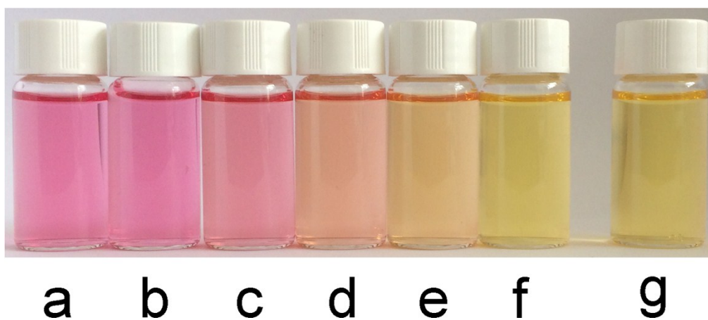
Fig. S5 Color photographs of xylene orange solution 2 at pH 5 in the presence of 20 \mu\text{M} (a), 15 \mu\text{M} (b), 10 \mu\text{M} (c), 5 \mu\text{M} (d), 1 \mu\text{M} (e), 0 \mu\text{M} (f) of Gd(III) ion and 1mM Gd chelates ( GdL_1 ) (g), respectively. The concentration of xylene orange solution is 12 mg/L.
