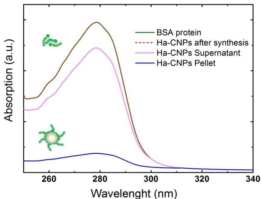
**Figure S4:** Absorption spectra of native biomolecule solution (green line), HA-CNPs samples directly after ablation (red dashed line), supernatant (magenta line) and pellet (blue line) after ultracentrifugation at 22,400 RCF. Compared to the protein absorption band prior to ablation, the peak intensity of protein was found to be nearly the same for HA-CNPs directly after ablation (red dashed line), indicating a high degree of molecule integrity.
