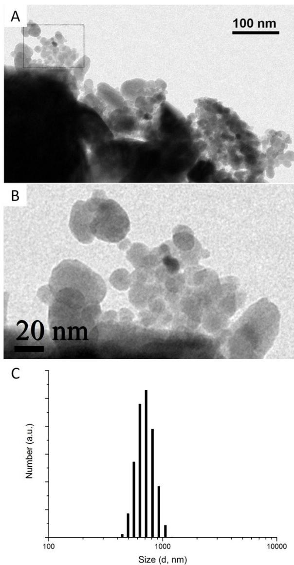
**Figure S2:** A) TEM observation of Ha-NPs colloidal solution prepared by infrared picoseconds laser ablation of HA target in deionized water; B) Magnification of the area signed with the black dashed line: it evidences that small nanoparticles are attached to each other in a cluster; C) DLS analysis of the as-synthesis Ha-NPs colloidal solution prepared in water exhibiting a mean size of  $(700 \pm 200)$  nm.
