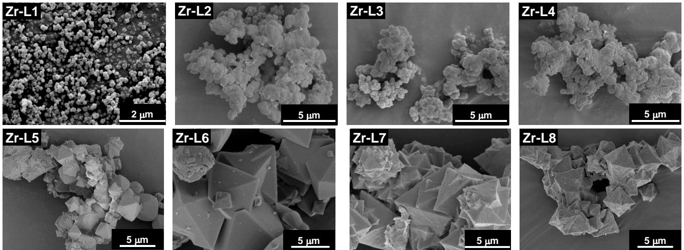
**Figure S2.** SEM images for Zr-based MOFs, Zr-L1 to Zr-L8.
