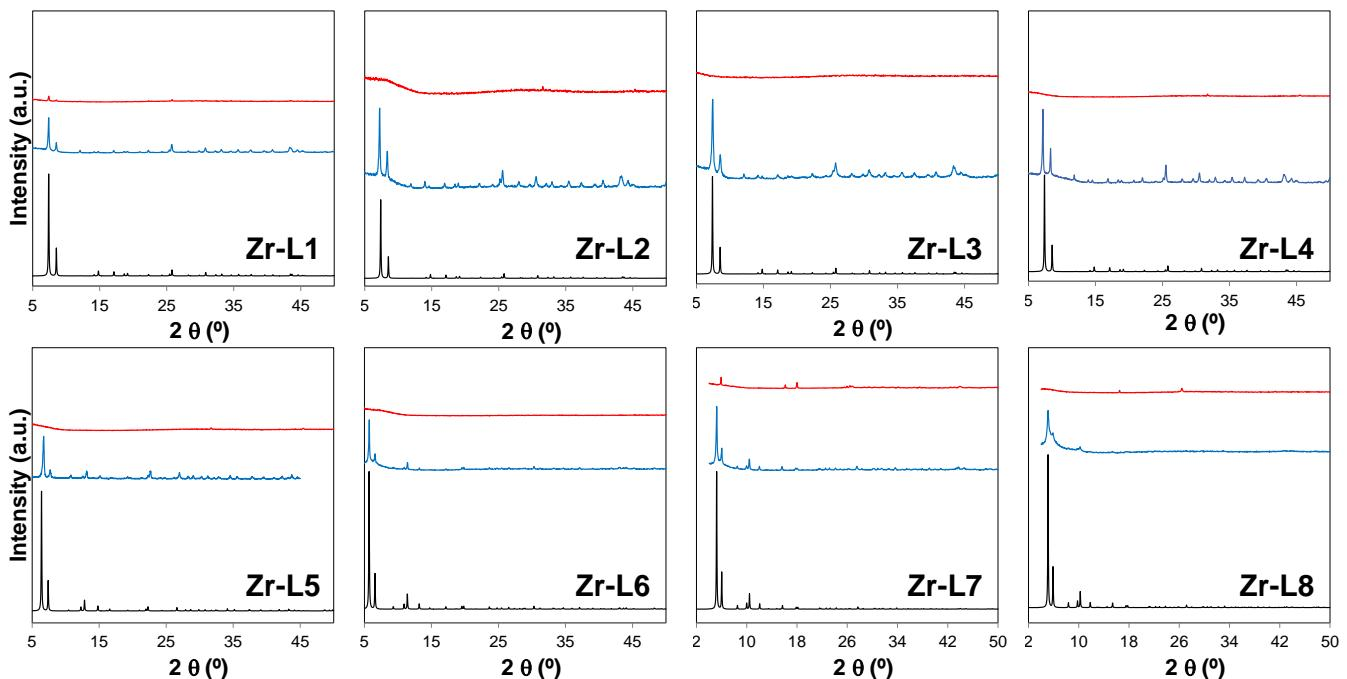
**Figure S6.** PXRD analysis of Zr-based MOFs after PBS exposure for 2 days. Color code of patterns: black, calculated; blue, synthesized; red, degraded after 2 days in PBS.
