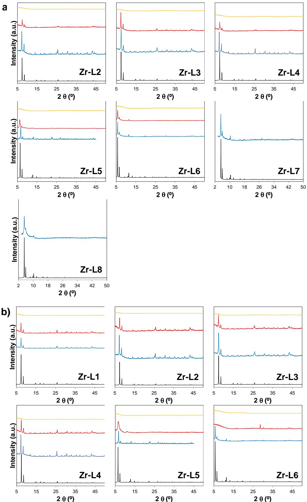
**Figure S1.** Powder X-ray diffraction (PXRD) patterns of synthesized Zr-based MOFs compared with the calculated pattern for each. Colour code of patterns: black, calculated; blue, synthesized; red, loaded; and, yellow, amorphized. a) calcein loaded materials and, b)  $\alpha$ -CHC loaded materials.
