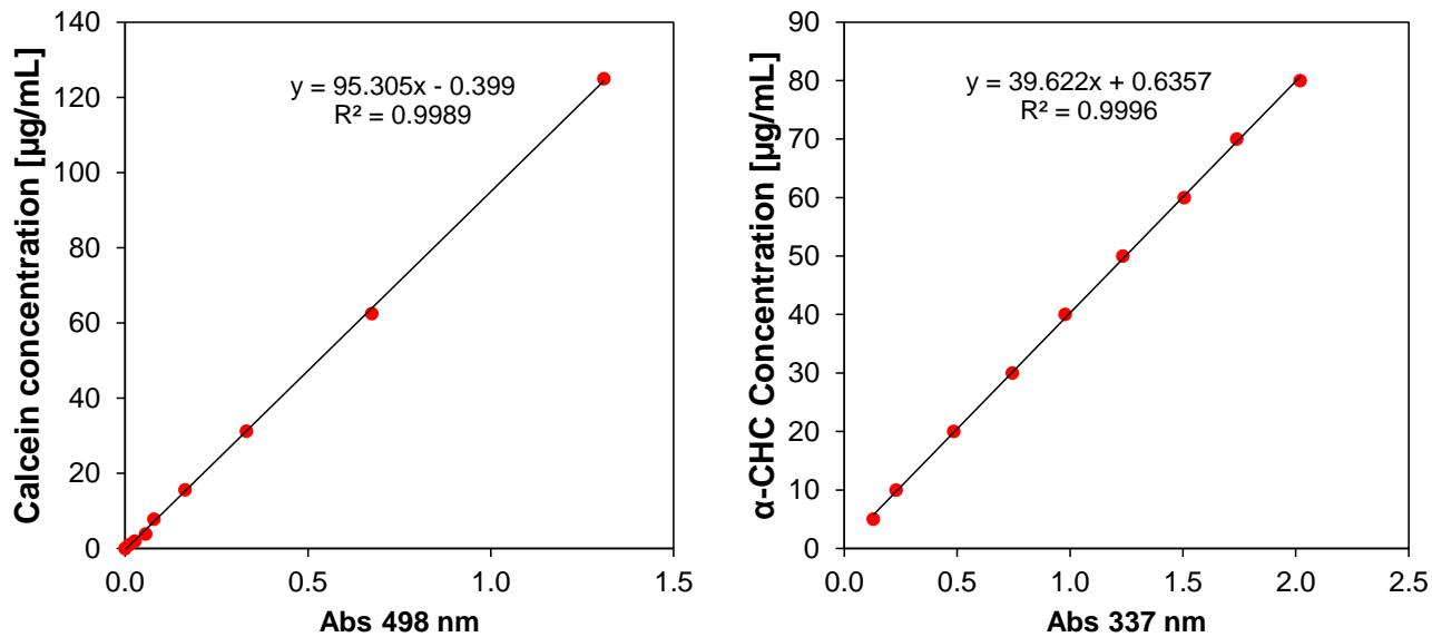
**Figure S15.** Calibration curve in PBS pH 7.4 for calcein (left) and  $\alpha$ -CHC (right) used for the release experiments.
