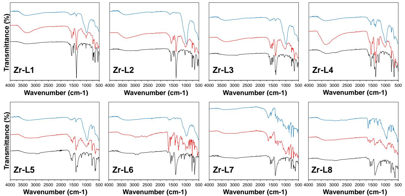
**Figure S7.** FTIR analysis of Zr-based MOFs after PBS exposure. Color code of patterns: black, no exposure to PBS; red, 2 days; and, blue, 3 days of PBS exposure.
