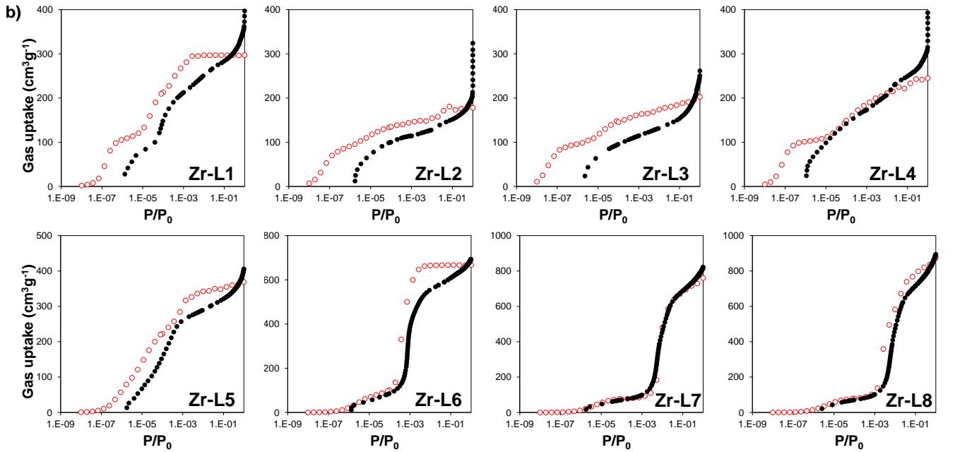
**Figure S3.**  $\text{N}_2$  adsorption isotherms for Zr-based family, experimental (black closed dots) and simulated (red opened dots). a) linear scale; b) semi-log scale.
