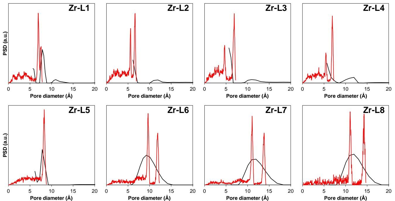
**Figure S4.** PSD analysis for Zr-based family, experimental (black continued line) and simulated (red continued line).
