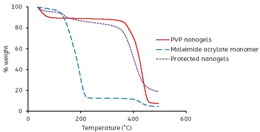
**Fig. S6** TGA thermograms of protected maleimide acrylate monomer, PVP nanogels and furan-protected maleimide-PVP nanogels
