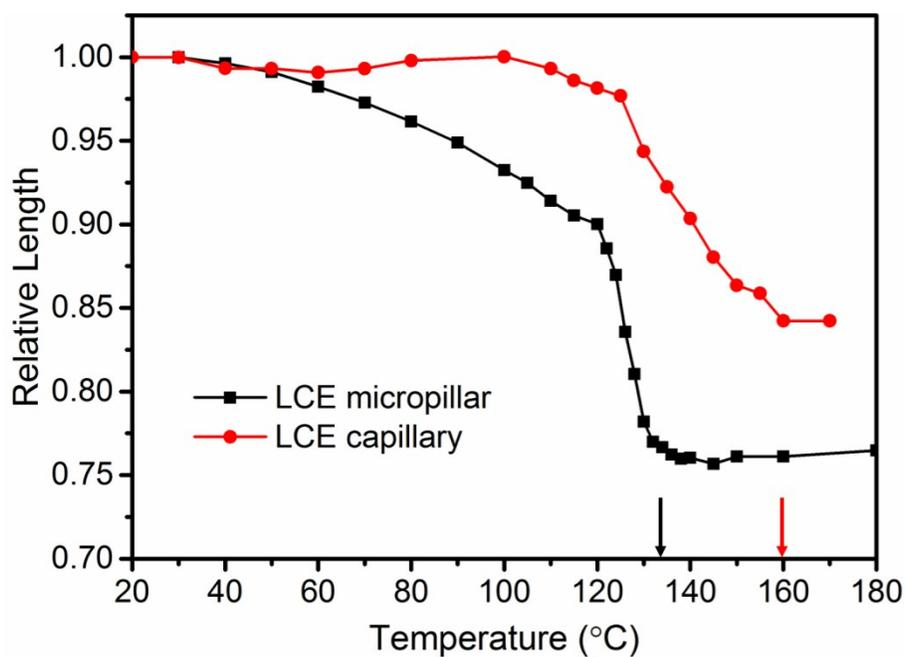
**Figure S2.** Temperature-dependent deformations of the LCE capillary and LCE micropillar. There is no residual polyimide layer on the micropillar surface, which was prepared by the method reported before.<sup>1</sup>
