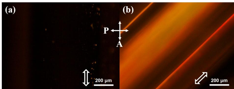
**Figure S1.** POM images of the tubular liquid crystal cell filled with aligned LCE precursor before photoinduced polymerization/crosslinking. The inserted white double-sided arrows represent the long axis directions (alignment direction) of the LC cells: (a) the alignment direction is parallel to the analyzer; (b) the alignment direction is 45° to the analyzer. P and A represent polarizer and analyzer, respectively.
