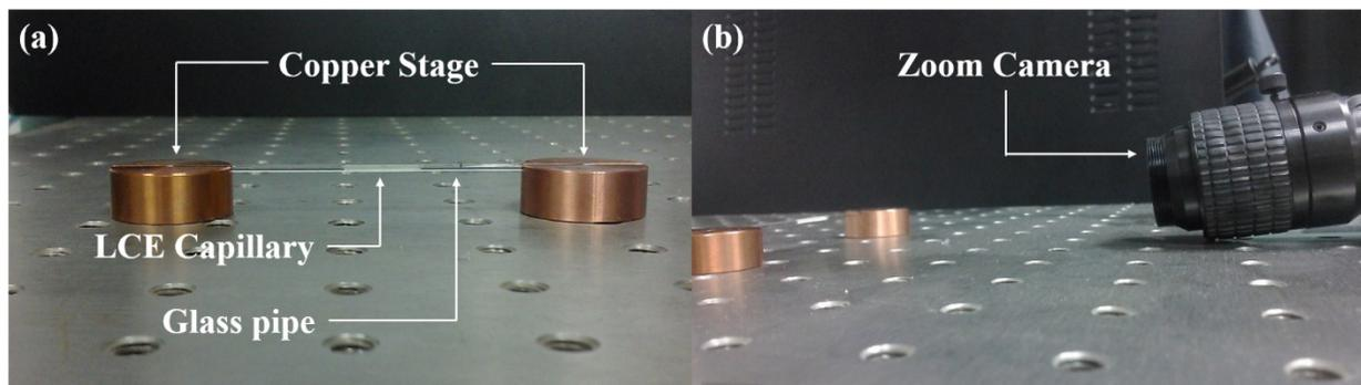
**Figure S3.** Experimental setup for investigating the LCE capillary peristaltic crawling locomotion. (a) Both ends of a glass tube with  $\sim 1$  mm inner diameter were immobilized on two copper stages, and the LCE capillary was placed in the glass tube. (b) Photographs and videos of the peristaltic crawling locomotion were recorded by a zoom CCD camera.
