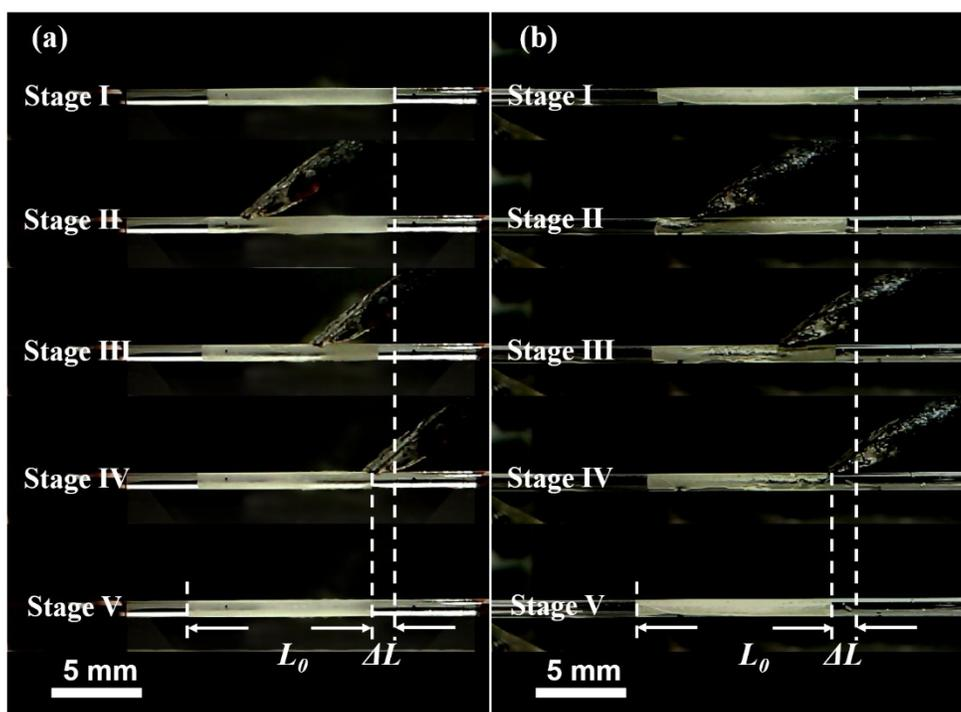
**Figure S4.** Peristaltic crawling for cases with or without the silicone oil: (a) the glass tube was fully filled with silicone oil; (b) no silicone oil was filled in the glass tube. The locomotion was observed for both cases with no obvious difference between them.
