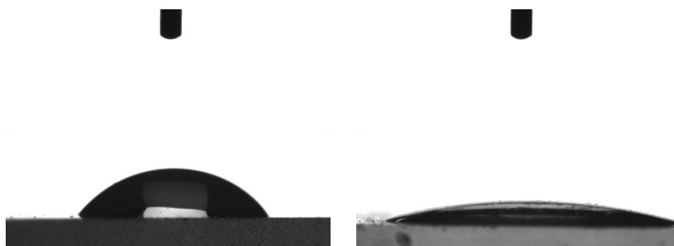
Figure S2 The water contact angel of glass slides before (left) and after (right) modification.
