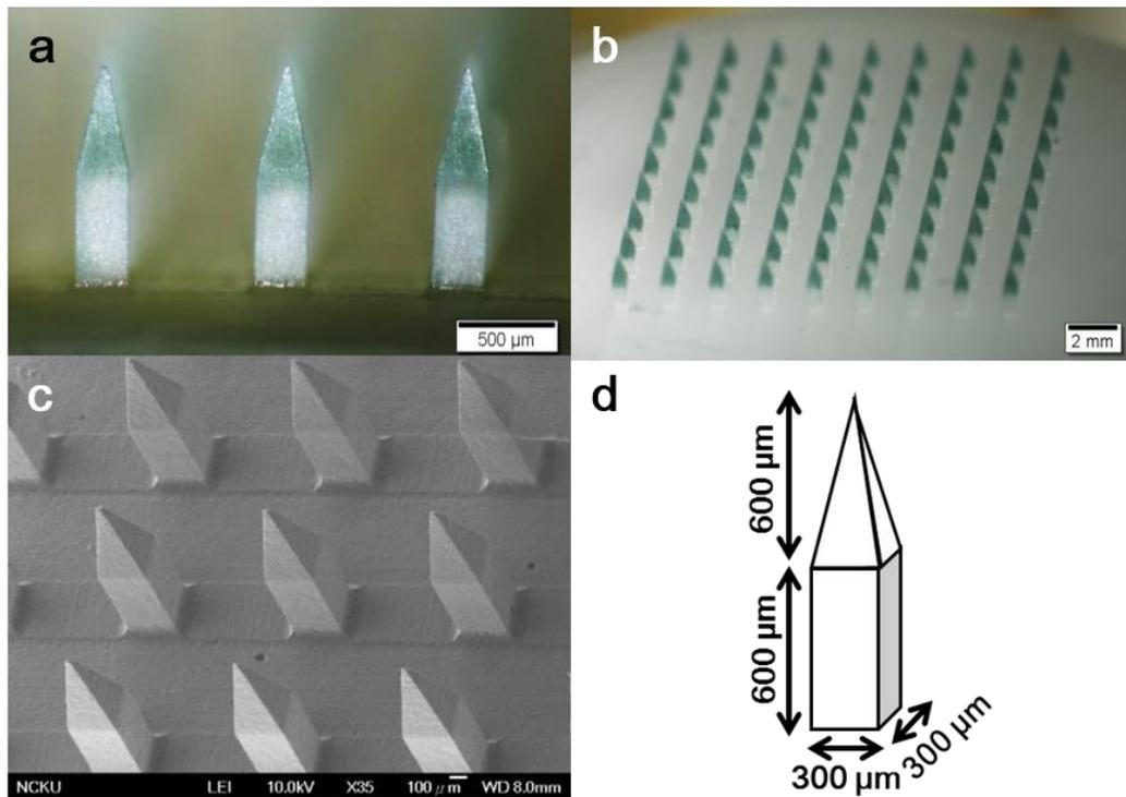
**Figure S1.** Characterization of nonimplantable MN system. This system consists of lidocaine-loaded polycaprolactone (PCL) MNs and a PCL supporting array patch. Bright-field micrographs (a and b), SEM image (c) and the detailed specifications of the needle (d).
