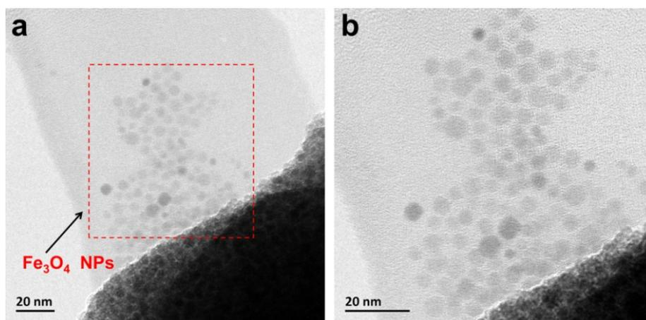
**Fig. S5** TEM images of HMS- $\text{Fe}_3\text{O}_4$  after dispersing in PBS media (pH 5.0) for 12 h, which indicating that free  $\text{Fe}_3\text{O}_4$  NPs were liberated from the nanosystem. Besides, the  $\text{Fe}_3\text{O}_4$  NPs are intact with no iron ions leakage in the *in vitro* pH 5.0 PBS media.
