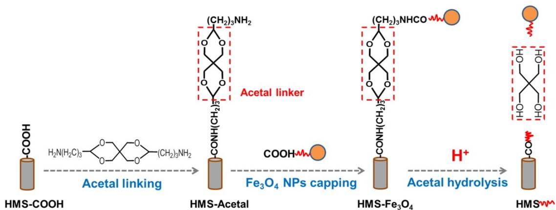
**Scheme S1** Illustration of the synthesis of HMS-Acetal and HMS-Fe<sub>3</sub>O<sub>4</sub>, and pH-responsive cleavage of the acetal linker in the HMS-Fe<sub>3</sub>O<sub>4</sub>.
