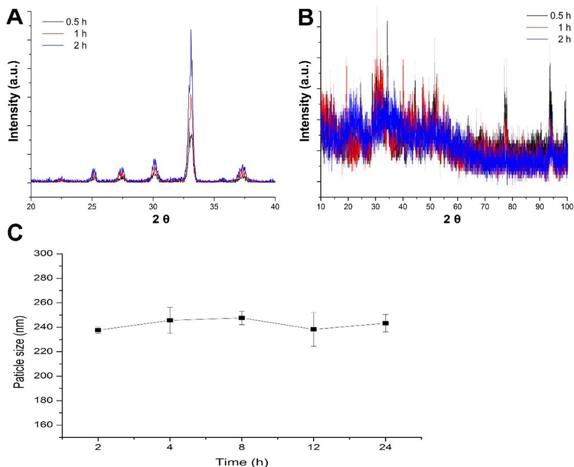
**Figure S2.** Comparative XRD patterns of ACC (A) and extractive OA-ACC core of PEG/OA-ACC (B) incubated with water for different time intervals (0.5, 1 and 2 h). (C) Stability tests of PEG/OA-ACC under physiological condition (PBS, pH 7.4) for 24 h. Results were expressed as mean  $\pm$  S.D. ( $n = 3$ ).
