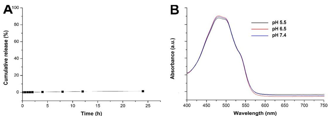
**Figure S3.** A) *In vitro* drug release of DOX from ACC-DOX in ethanol for 24 h. Results were expressed as mean  $\pm$  S.D. ( $n = 3$ ). B) UV spectra of the released DOX from ACC-DOX in various pH conditions (7.4, 6.5, and 5.5). When the ACC-DOX were charged into in aqueous solutions, the resulted solutions showed the featured absorption peak of DOX at 480 nm.
