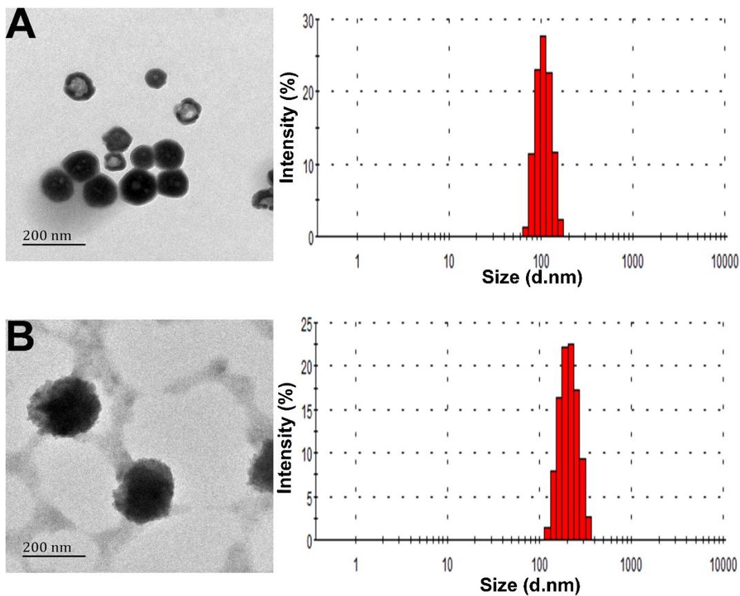
**Figure S4.** Representative TEM (left) and size distribution (right) images CCC-DOX (A) and PEG/OA-CCC-DOX (C). Scale bars: 200 nm.
