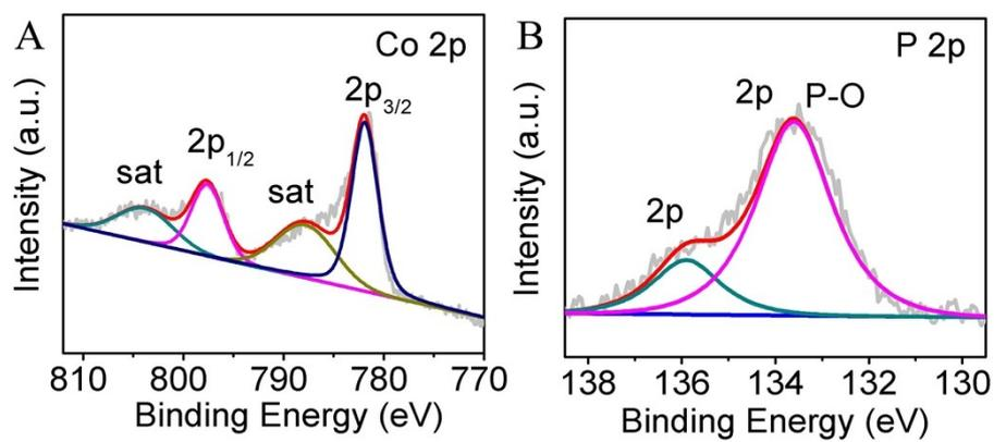
**Fig. S1.** XPS spectra of (A) Co 2p and (B) P 2p for CoP NA after potential cycling in 0.1 M NaOH.
