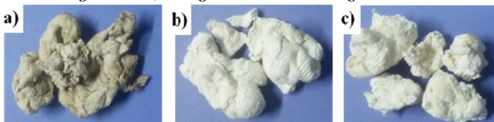
Fig. S9 Photo images of a) PVA-g-DBA/BA, b) PVA-g-DMB/BA and c) PVA-g-PHB/BA. For the PVA-g-DMB/BA and PVA-g-PHB/BA, no color change was observed before (b and c) and after ( Figure 4c B and C ) curing.
