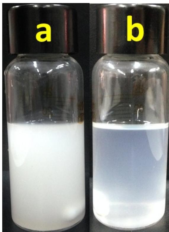
**Figure S2.** Photographs of aqueous solutions of (a) mesoporous silica shells coated ZIF-8 (ZIF-8@MSN); (b) ZIF-8@MSN after dilute HCl etching to produce HMSN.
