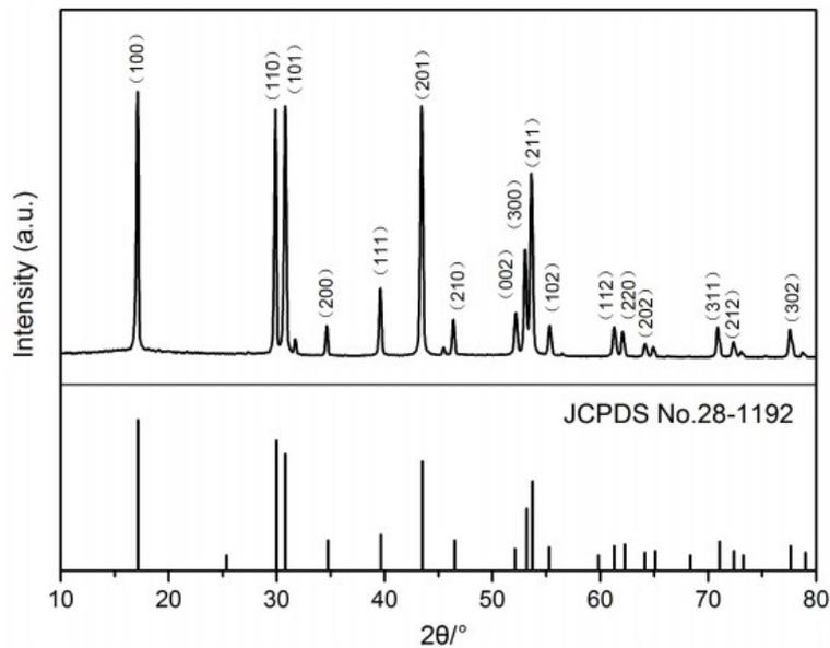
**Fig. S2** The powder X-ray diffraction (XRD) pattern of oleic acid-capped NaYF<sub>4</sub>:Yb<sup>3+</sup>/Er<sup>3+</sup> NPs and the standard pattern of hexagonal NaYF<sub>4</sub> (JCPDS No.28-1192).
