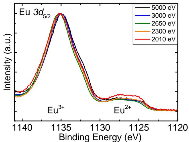
**Fig. 1** HAXPES spectra of the Eu  $3d_{5/2}$  core level of a sample grown under the Eu distillation condition. Spectra normalized to the  $\text{Eu}^{3+}$  component.
