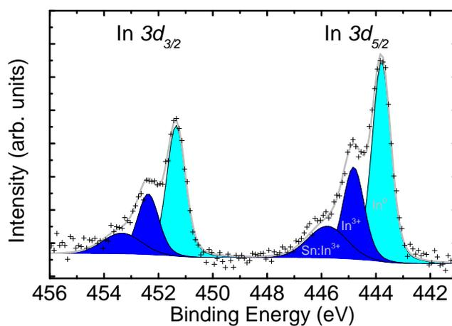
**Fig. 4** HAXPES spectrum of the In  $3d$  core level of sample type (iii). Spectrum recorded with a photon energy of 2010 eV.  $\text{In}^{3+}$  components are shown in dark blue,  $\text{In}^0$  in light blue. Black crosses represent the experimental data, gray line is the superposition of all fit components.
