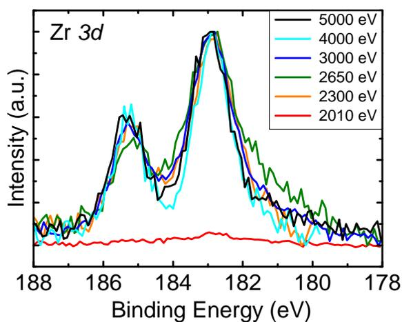
**Fig. 2** HAXPES spectra of the Zr  $3d$  core level of sample type (ii) discussed in the manuscript. Spectra normalized to the Zr  $3d_{5/2}$  components, except for the 2010 eV spectrum which could not be normalized because the intensity is too weak.
