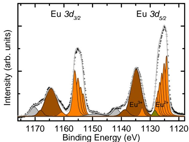
**Fig. 3** HAXPES spectrum of the Eu  $3d$  core level of sample type (iii). Spectrum recorded with a photon energy of 5000 eV.  $\text{Eu}^{2+}$  components are shown in orange,  $\text{Eu}^{3+}$  in brown, and plasmonic excitation in gray. Black crosses represent the experimental data, gray line is the superposition of all fit components.
