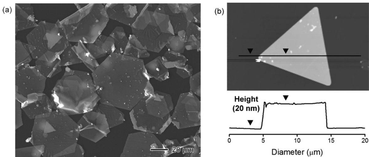
**Fig. S1** (a) Scanning electron microscopy (SEM) image of Au nanosheets. (b) Atomic force microscopy (AFM) image of a single Au nanosheet, showing its thickness of about 20 nm.
