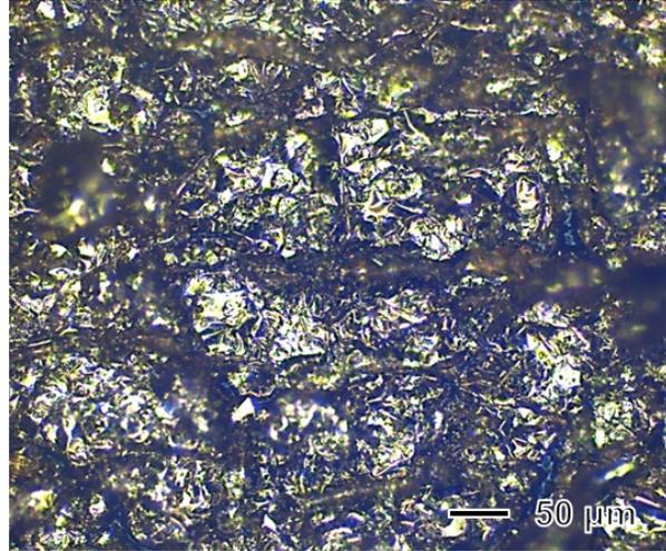
**Fig. S4** OM image of eight-layer Au nanosheet film on Ecoflex substrate taken after 10,000 cycles of stretching at  $\varepsilon = 0.5$ .
