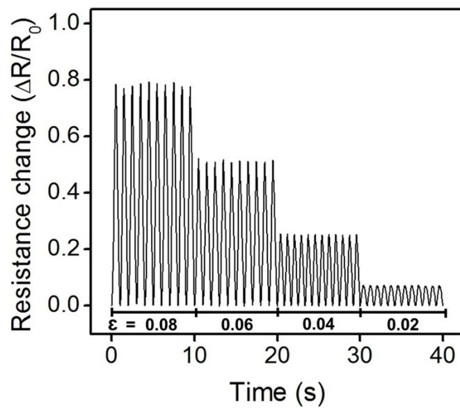
**Fig. S7** Time-dependent  $\Delta R/R_0$  of the sensor based on bilayer Au nanosheet film in response to repetitive stretching at strains from 8 to 0% with decrement of 2% (10 cycles per strain).
