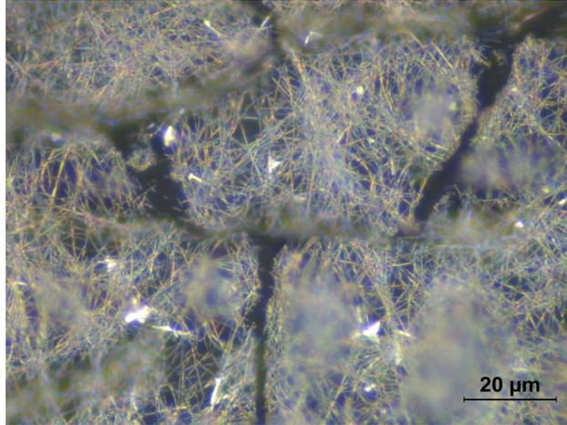
**Fig. S3** OM image of Ag nanowire film on Ecoflex substrate taken after 10,000 cycles of stretching at  $\varepsilon = 0.5$ , showing the generation of cracks in the film.
