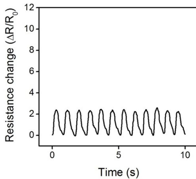
**Fig. S8**  $\Delta R/R_0$  response of the sensor shown in Fig. 4d measured after 1,500 steps of walking.
