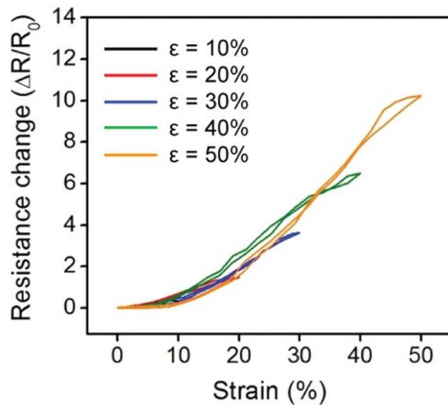
**Fig. S6** Hysteresis curves of the eight-layer Au nanosheet film measured at different strains.
