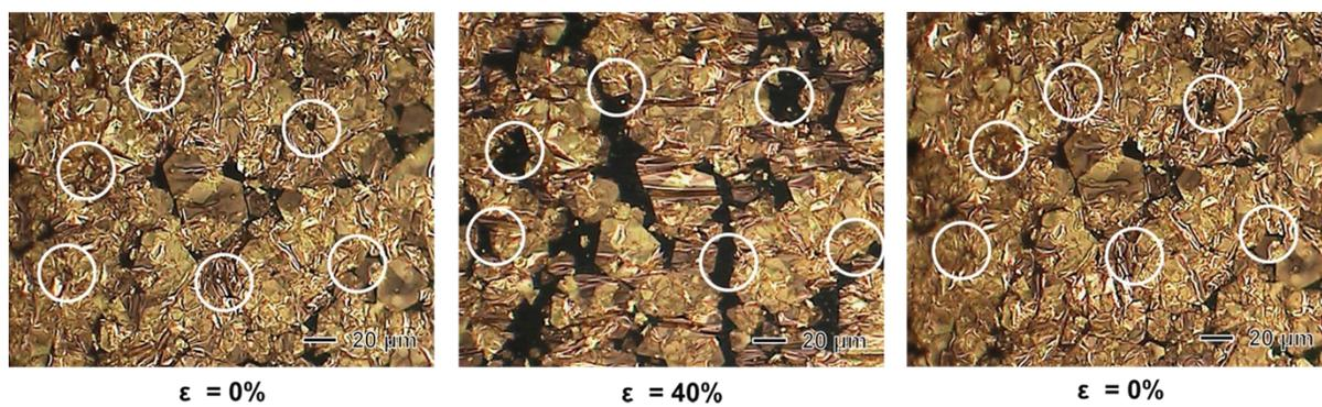
**Fig. S5** OM images showing the reversible sliding of Au nanosheets during a stretching and releasing cycle.
