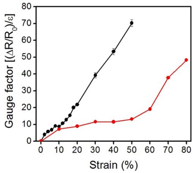
**Fig. S2** Gauge factors of Au nanosheet strain sensors based on bilayer (black line) and eight-layer (red line) Au nanosheet films according to tensile strain.
