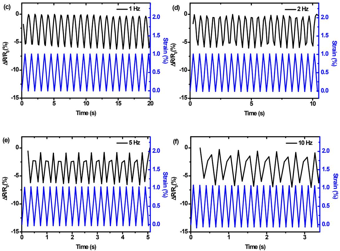
**Figure S8.** The relative resistance change of GNWF sensor with 1 % strain under various frequencies (a) 0.1 Hz, (b) 0.5 Hz, (c) 1 Hz, (d) 2 Hz, (e) 5 Hz and (f) 10 Hz.
