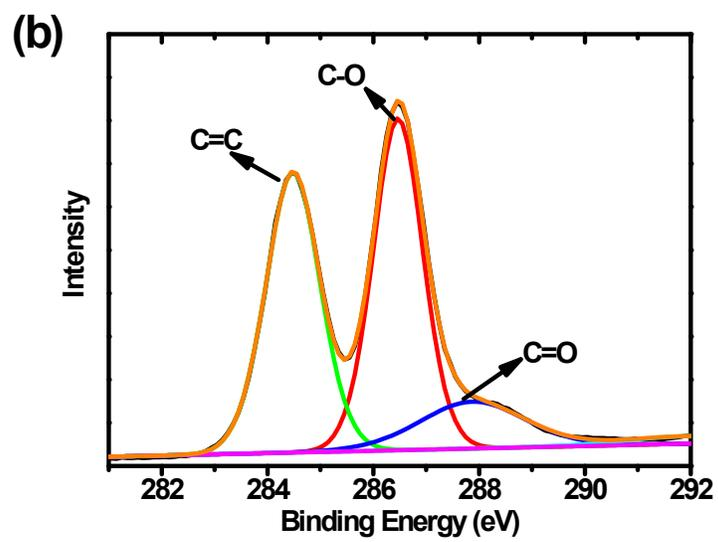
**Figure S1.** (a) AFM image of GO sheets on a silicon substrate, (b) XPS C1s spectrum of GO.
