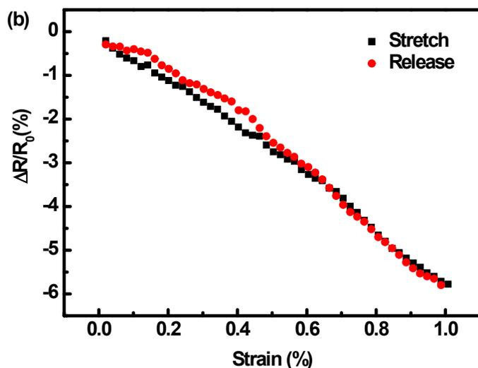
**Figure S7.** (a) The relative resistance change of GNWF sensor with 1 % strain over 10000 cycles. (b) The relative resistance change of GNWF sensor during stretching and relaxation.
