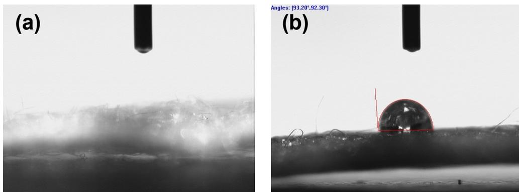
**Figure S2.** Water drop contact angles on (a) NWF and (b) GNWF.
