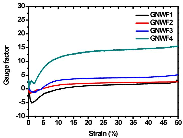
Figure S6. Calculated gauge factor of GNWFs change with strain.
