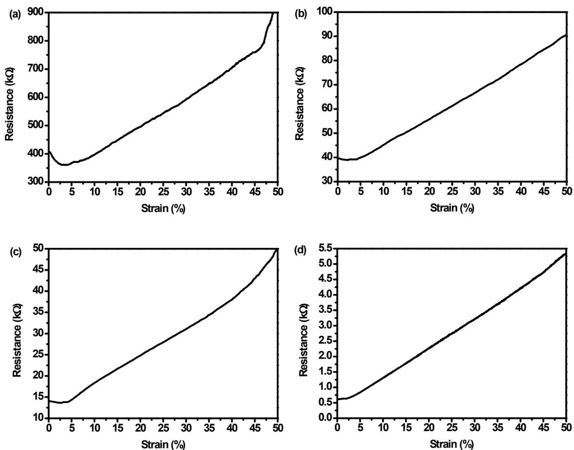
**Figure S5.** Resistance change of (a) GNWF1, (b) GNWF2, (c) GNWF3 and (d) GNWF4 with applied tensile strain.
