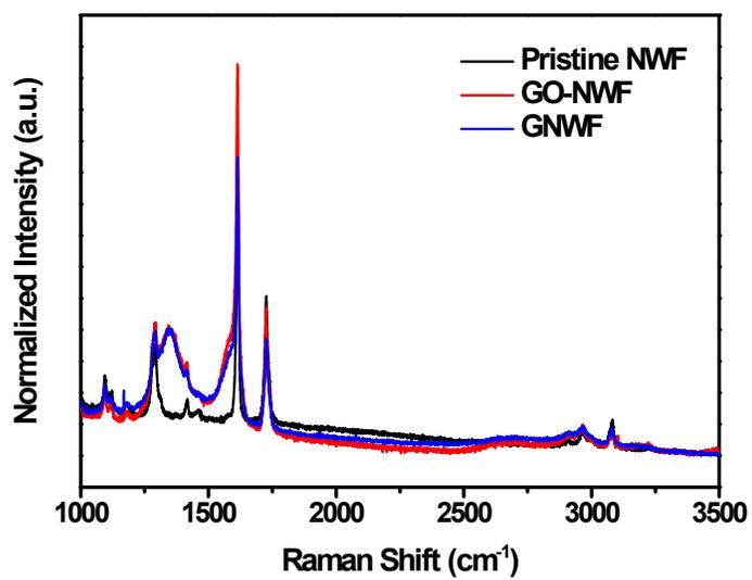
**Figure S3.** Raman spectra of pristine, GO coated and reduced GO coated NWFs.
