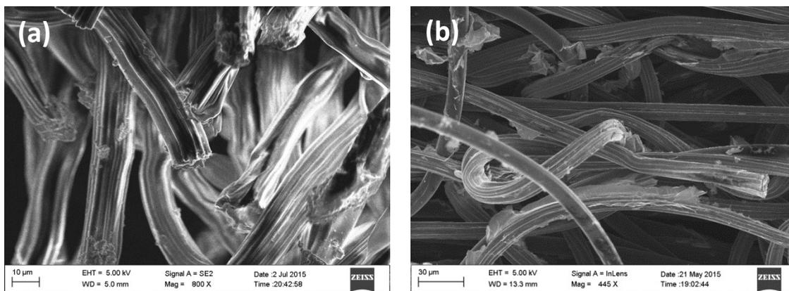
**Figure S4.** SEM image of (a) pristine NWF and (b) GNWF4 (rGO loading 2.3 wt.%)
