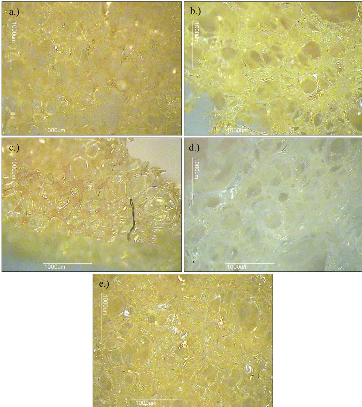
**Figure S5:** Micrographs of a.) non-poled sample, b.) 150 V, c.) 500 V, d.) 1051 V, and 2000 V poled samples.
