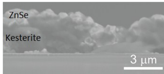
Figure SI4: SEM cross section image of a sister sample prealloyed and annealed in the same conditions than the reference sample.
