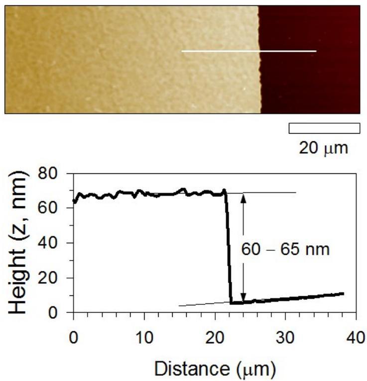
**Figure S5.** AFM topography (top) and cross-section profile (bottom) of the 100- $\mu\text{m}$  patterned TES-ADT film.
