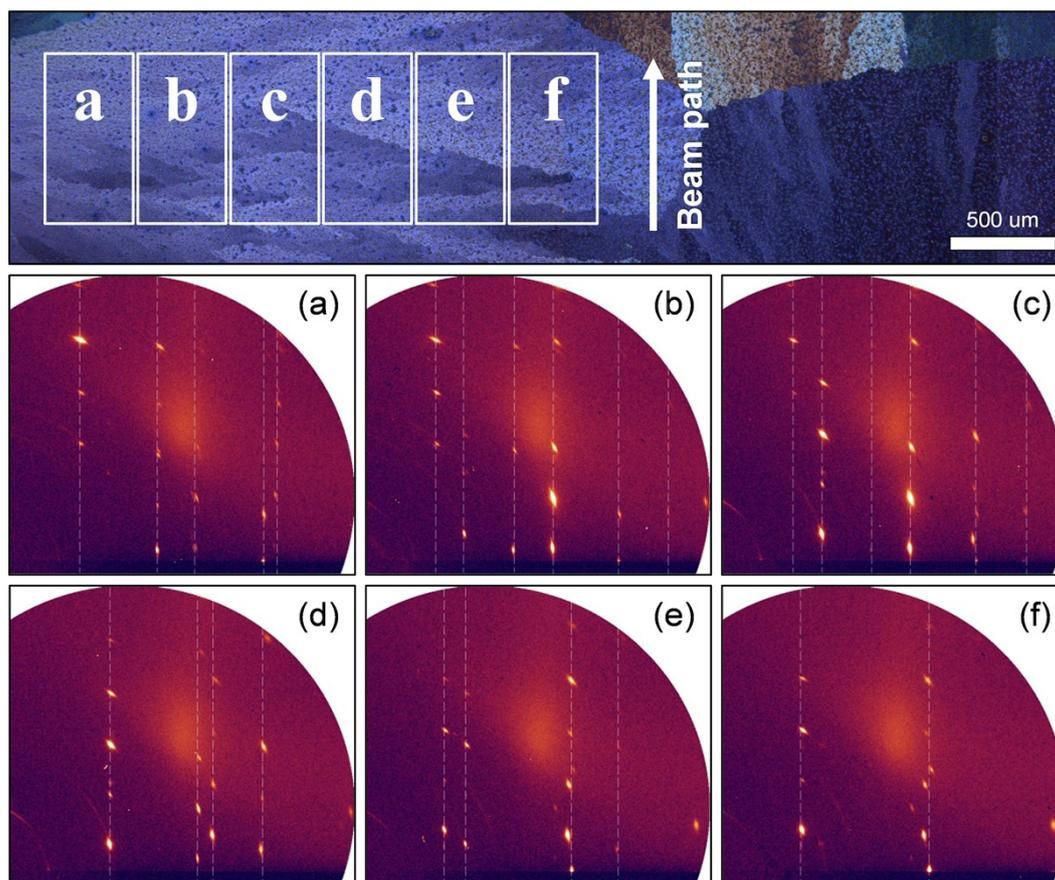
**Figure S9.** 2D GIXD patterns obtained from a normal DSA-treated TES-ADT film along the footprint of the incident beam with a width  $\times$  height of  $300 \times 50 \mu\text{m}^2$ . The patterns corresponding to each footprint are indicated in the upward-polarized OM images.
