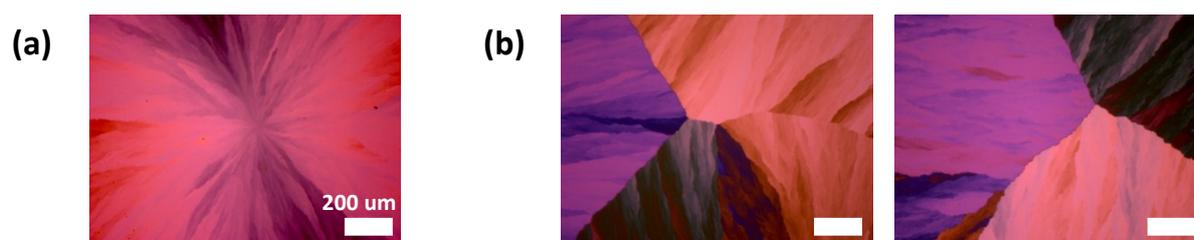
**Figure S3.** Polarized OM images of the unpatterned TES-ADT films after applying the solvent annealing process.
