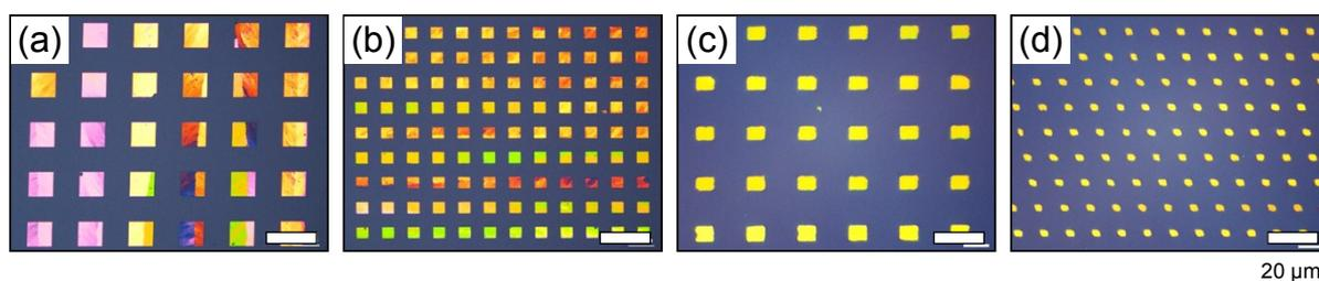
**Figure S4.** Polarized OM images of square-patterned TES-ADT films prepared using (a) 100, (b) 50, (c) 10, (d)  $2.5 \mu\text{m}$  line patterned PDMS stamps.
