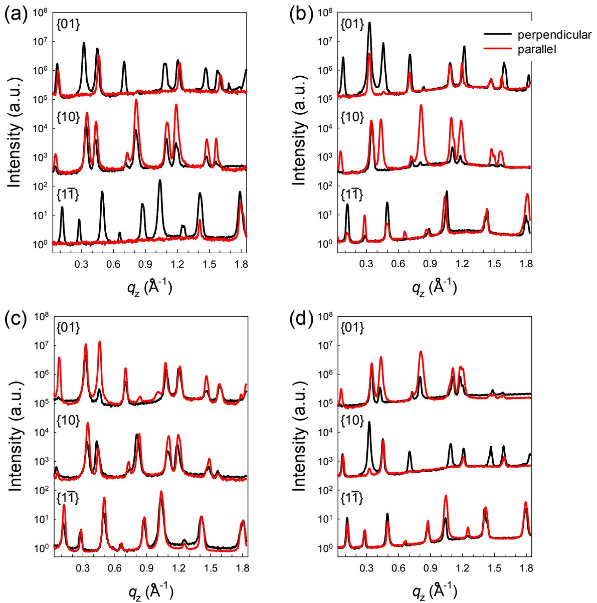
**Figure S8.** 1D X-ray reflections extracted at  $q_{\{01\}}$ ,  $q_{\{10\}}$ , and  $q_{\{1\bar{1}\}}$  from the 2D GIXD patterns of (a) 100, (b) 50, (c) 10, (d) 2.5  $\mu\text{m}$  TES-ADT samples (Figure 5).
