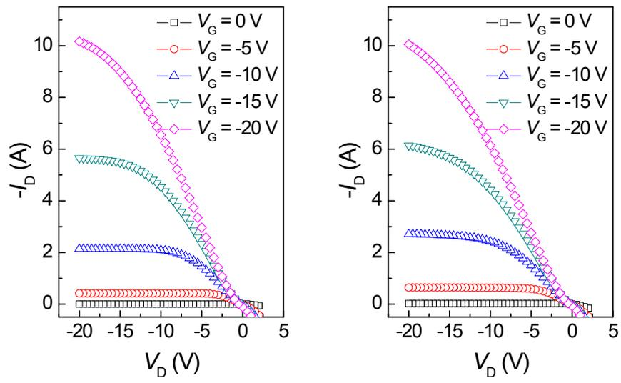
**Figure S10.** Output characteristics of OFETs prepared with 100 or 2.5  $\mu\text{m}$ -patterned TES-ADT film.
