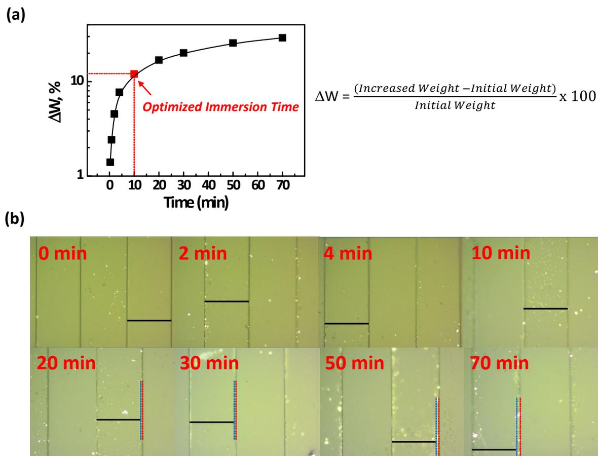
**Figure S1.** (a) Degree of weight increase and (b) OM images of the 50  $\mu\text{m}$ -patterned PDMS stamp over time during immersion in the DCE reservoir. Note that in (b), the black scale bars indicate 50  $\mu\text{m}$ . As the immersion time increased, particularly after 10 min, the line width of the PDMS stamp increase, indicating swelling in the PDMS.
