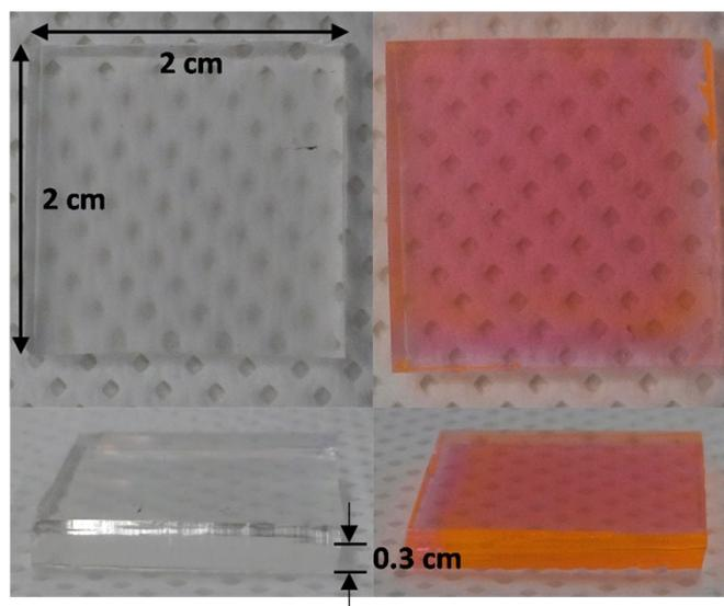
**Figure S2.** Photographs of the  $\mu$ -PDMS stamps before and after the TES-ADT patterning process.
