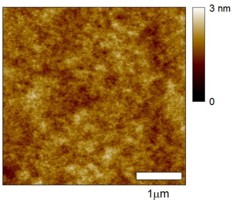
**Figure S6.** 2  $\mu\text{m}$   $\times$  2  $\mu\text{m}$  AFM topography image of the as-spun TES-ADT film.
