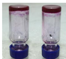
Figure S2. Pictures of the gels of ABVA (left) and AVBVA (right) obtained from 1,4-dioxane/cyclohexane (v/v = 1/4).
