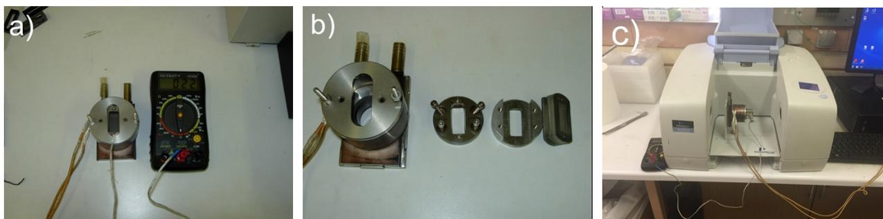
**Figure S14.** Set-up used to record the FTIR behavior of **5** as a function of the temperature. **5** was disposed in a screw sealed cell built from two slices of crystalline KBr. It was deposited by drop casting between two KBr Slices. a) KBr sealed cell; b) KBr opened cell; c) KBr sealed cell disposed in the Perkin-Elmer Spectrum 100 FT-IR spectrometer.
