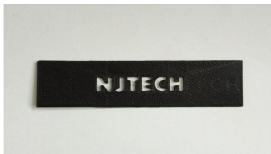
Fig. S1 A mask patterned with “NJTECH” obtained by a 3D printer
