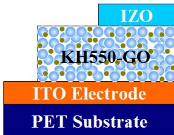
Figure S2. An ITO/KH550-GO/IZO sandwich structure for testing the proton conductivities and the specific capacitance
