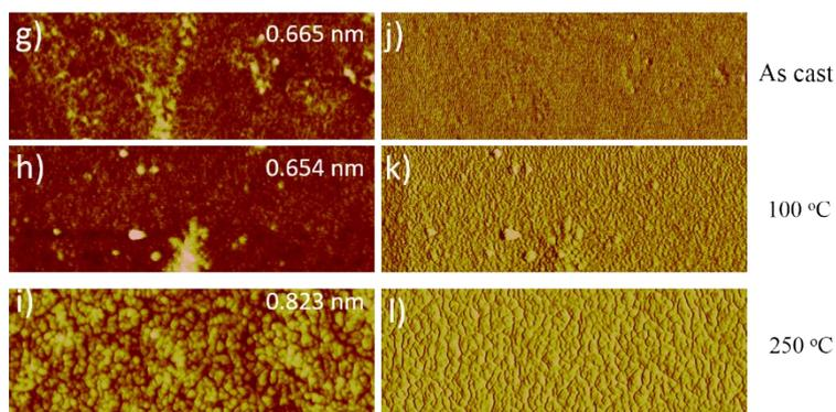
**Figure S7:** AFM topography (a,b,c) and phase (d,e,f) images of **PAIDBT**, and AFM topography (g,h,i) and phase (j,k,l) images of **PAIDSe**, as cast and after annealing at 100 °C and 250 °C. Scan size: 5  $\mu\text{m}$   $\times$  5  $\mu\text{m}$ .
