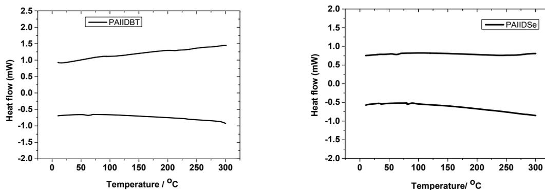
**Figure S2:** DSC traces of **PAIIBDT** and **PAIDSe** recorded at 10 °C /min from 0 to 300 °C (the tiny peaks of both polymers are from instrument artefact).
