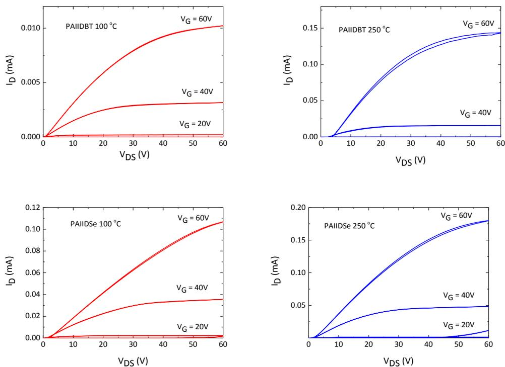
**Figure S6:** Output characteristics of **PAIIDBT** (a, b) and **PAIIDSe** (c, d) annealed at 100 °C and 250 °C.
