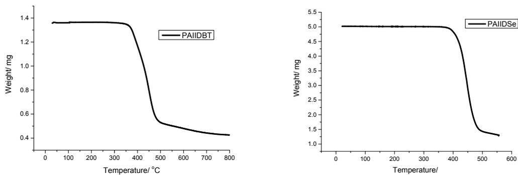
**Figure S1:** Thermal gravimetric analysis (TGA) of polymer **PAIIBDT** (Td: 375 °C) and **PAIDSe** (Td: 410 °C) recorded at 30 °C /min in a nitrogen atmosphere.
