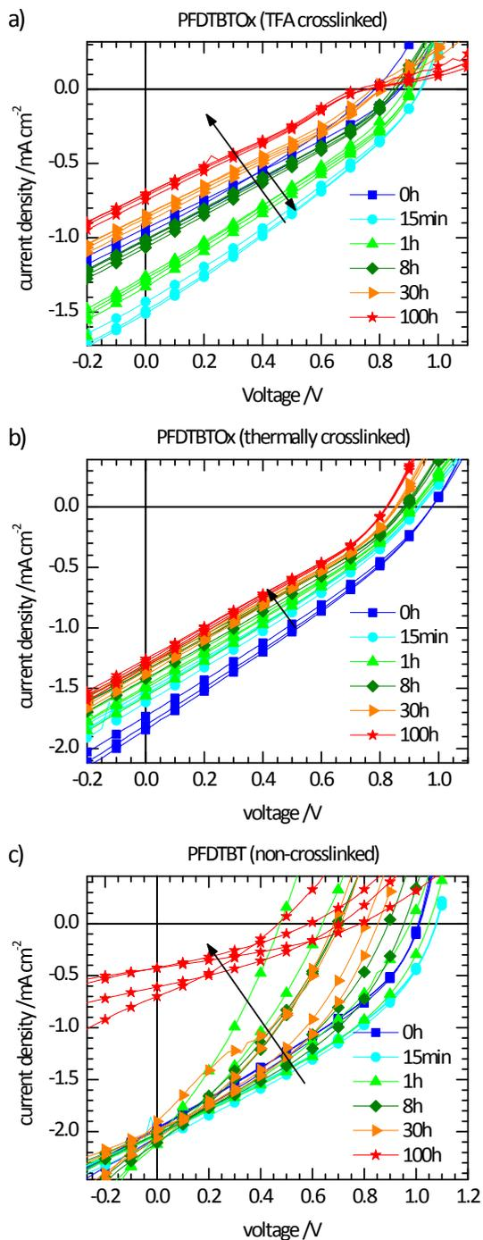
**Figure S 6.**  $J$ - $V$  characteristics from accelerated aging tests of the TFA crosslinked PFDTBTOx (a), thermally crosslinked PFDTBTOx (b), and non-crosslinkable PFDTBT (c) in a polymer:PCBM blend with a 1:2 ratio. For each material combination four solar cells were measured.
