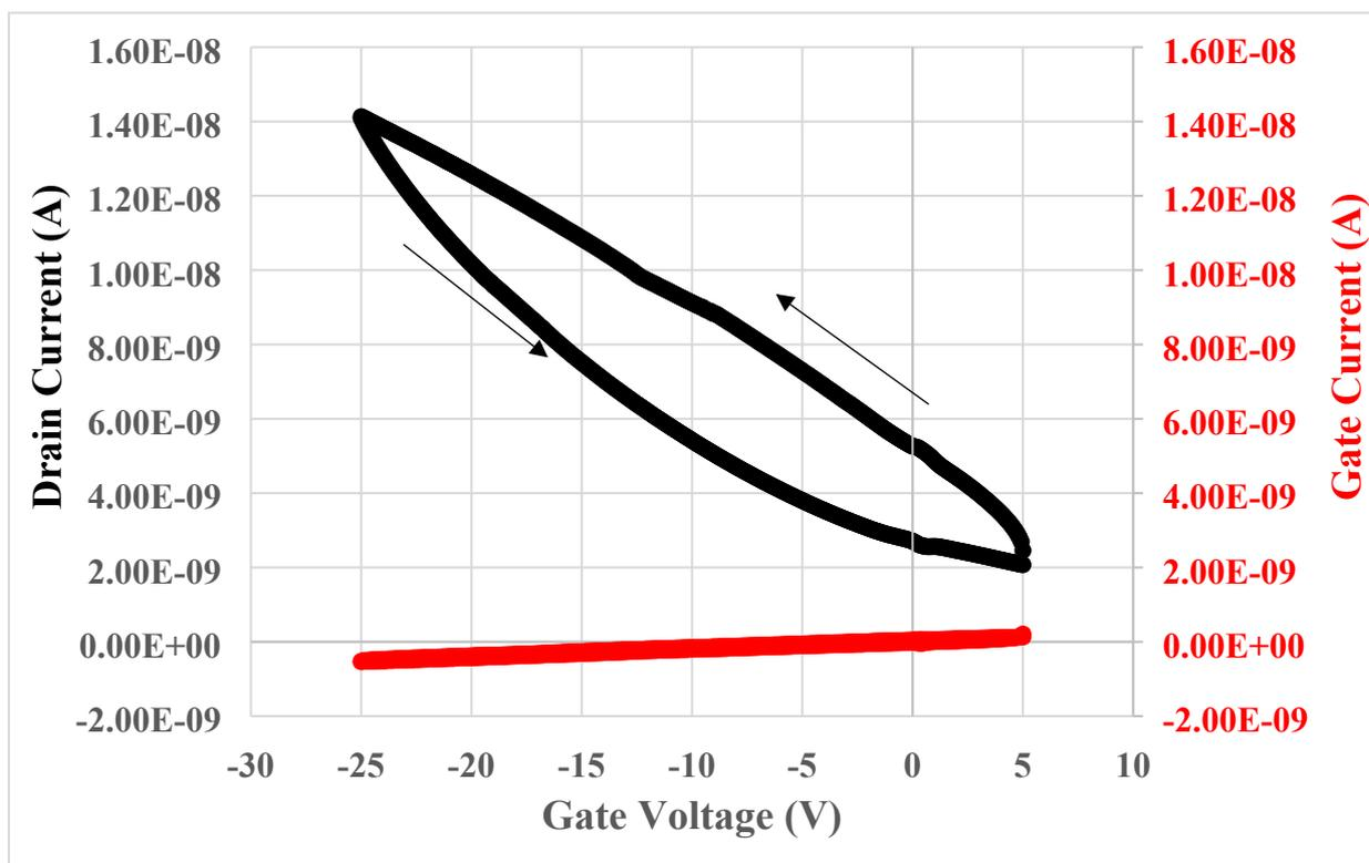
Figure S2. Characterization of CuI TFTs printed at 60 °C: (a) output characteristic curves, (b) hysteresis and gate leakage current measurement.
