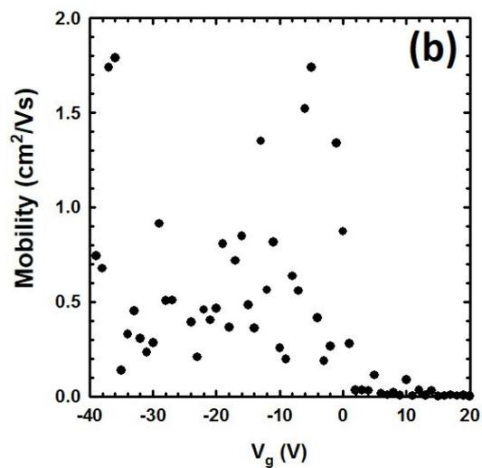
Figure S1. Mobility values of (g) printed CuI TFTs at room temperature and (h) printed CuI TFTs at 60 °C as a function of gate voltage.
