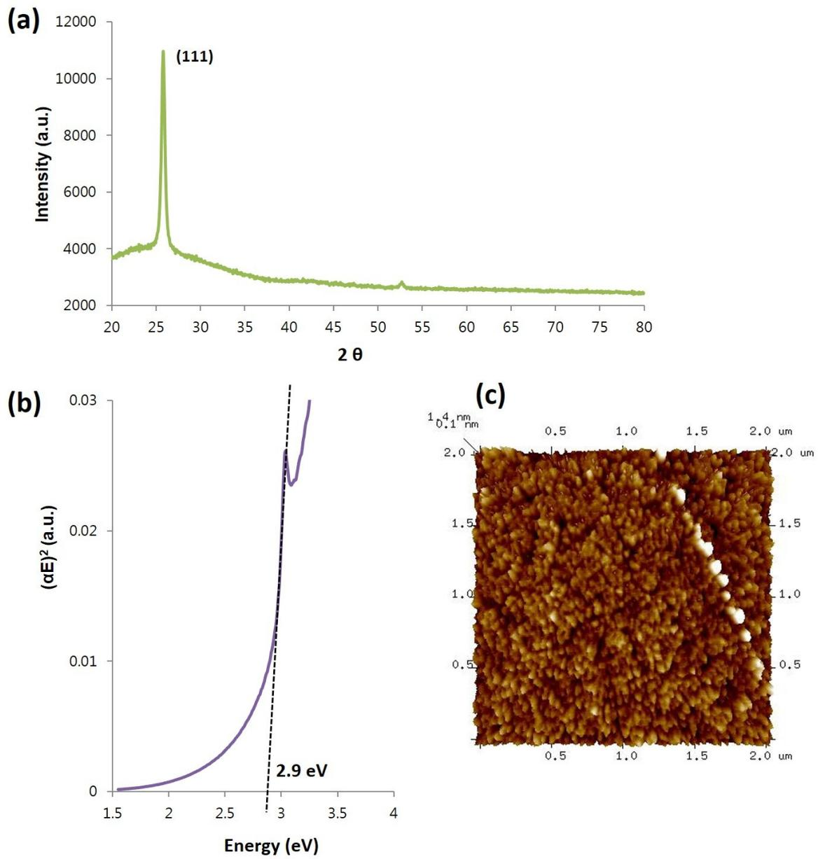
Figure S3. Characterization of printed CuI TFTs baked at 150 °C: (a) XRD pattern, (b) band gap measurement, and (c) AFM image.
