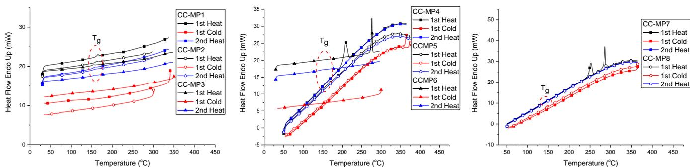
**Fig. S2** DSC curves for CC-MP compounds (after heated at 110 °C for 1h) at a scan rate of 10 °C/min.
