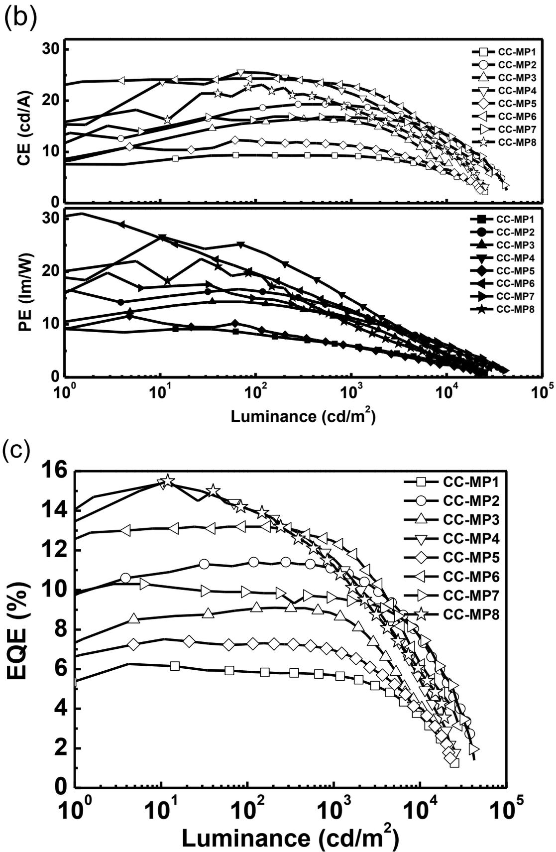
Fig. S12 J-V-L (a), CE-L-PE (b), EQE-L (c) plots of the OLED device.
