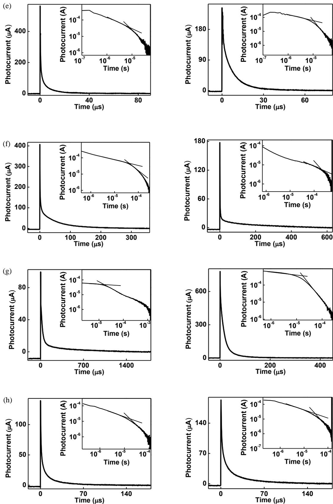
**Fig. S10** The representative TOF transients for electrons (left) and holes (right) of **CC-MP1** (a), **CC-MP2** (b), **CC-MP3** (c), **CC-MP4** (d), **CC-MP5** (e), **CC-MP6** (f), **CC-MP7** (g), and **CC-MP8** (h).
