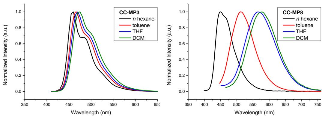
**Fig. S3** PL spectra of CC-MP3 and CC-MP8 in different solvents.
