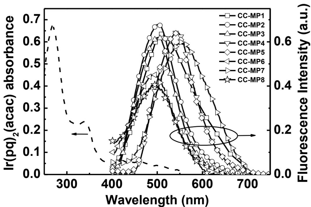
Fig. S11 Film PL spectra of selected CC-MP dyes and absorption spectrum of Ir(pq)<sub>2</sub>(acac).
