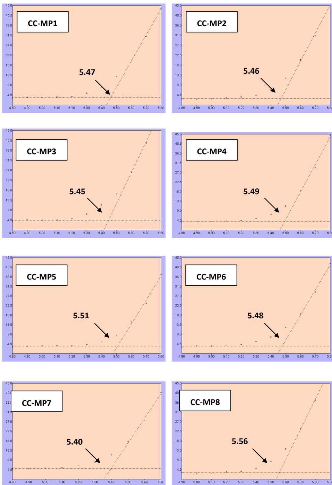
Fig. S5 Low-energy photoelectron spectra of all compounds.
