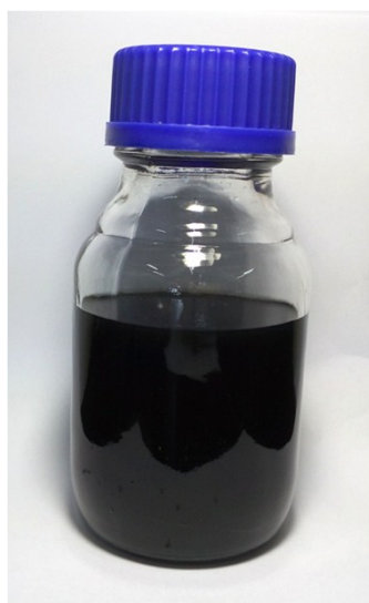
Fig. S1 Photo of ethanol-assisted dispersed CNTs suspensions.
