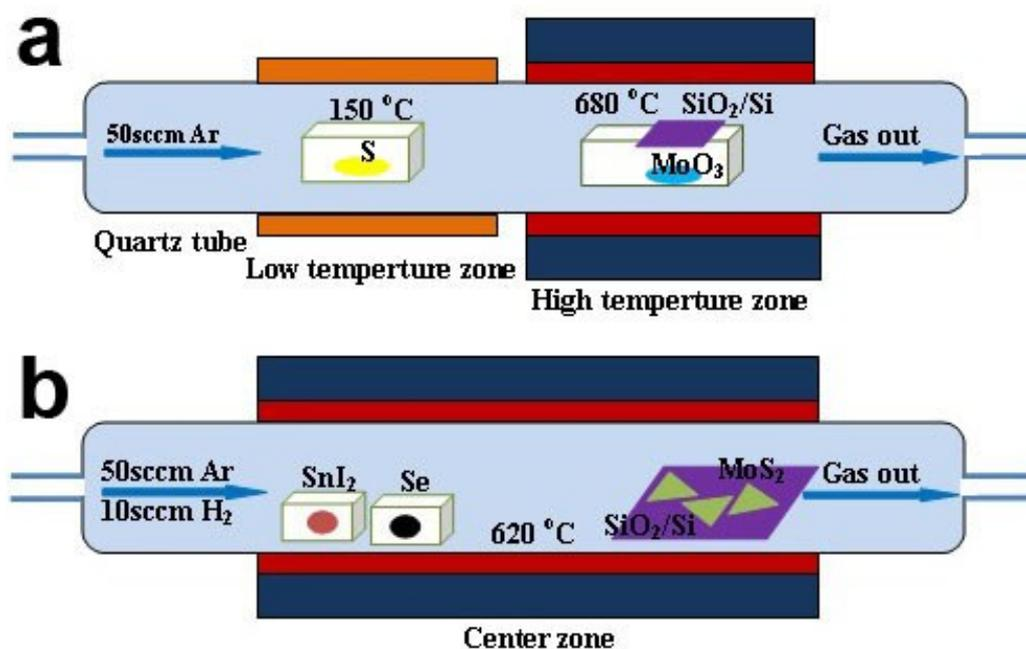
Figure S1 Schematic illustration of the CVD system for the growth of (a) Monolayer MoS<sub>2</sub> triangular sheets and (b) SnSe<sub>2</sub>/MoS<sub>2</sub> heterostructures.
