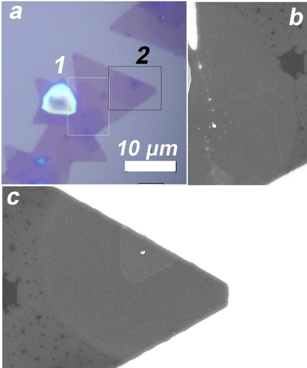
Figure S2 (a) Optical microscope image of the SnSe<sub>2</sub>/MoS<sub>2</sub> heterojunctions. (b, c) Enlarged view of SEM images (SEI mode) of the area indicated by white rectangle and black rectangle, respectively. We can see the layer-by-layer stacking structures in the SEM images (SEI mode).
