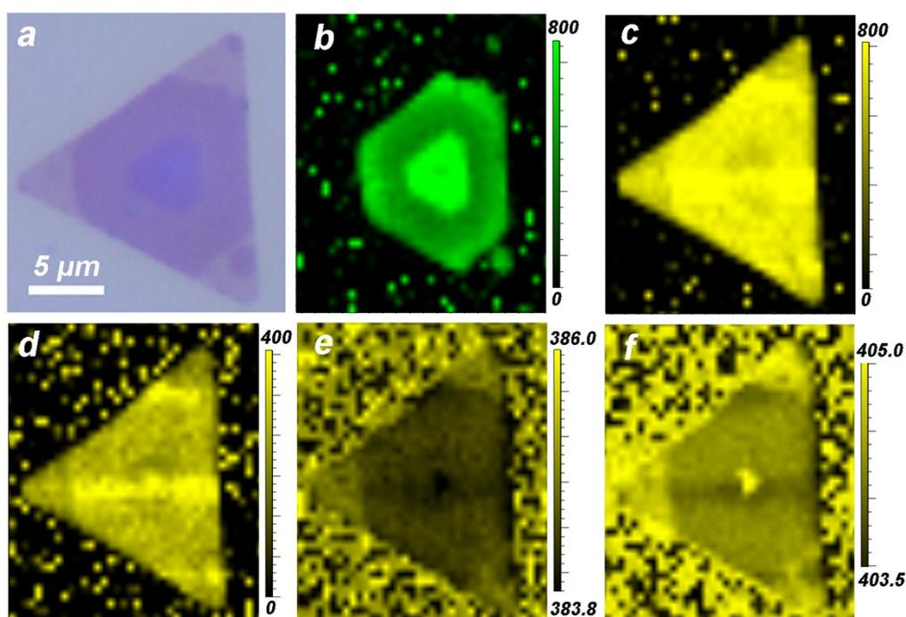
Figure S5 (a) An optical microscope image of a triangular MoS<sub>2</sub> monolayer covered partially with a SnSe<sub>2</sub> multilayer. Spatially resolved Raman maps for the intensity of A<sub>1g</sub> of SnSe<sub>2</sub> (b), A<sub>1g</sub> of MoS<sub>2</sub> (c), E<sup>1</sup><sub>2g</sub> of MoS<sub>2</sub> (d), and the peak position of E<sup>1</sup><sub>2g</sub> of MoS<sub>2</sub> (e), A<sub>1g</sub> of MoS<sub>2</sub> (f).
