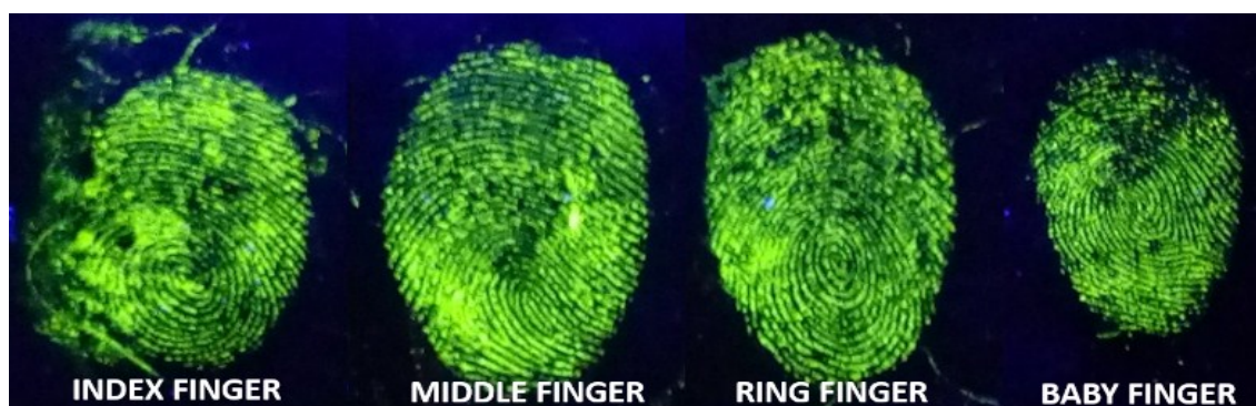
Figure S20 Fluorescence images of 24 h aged fingerprints of all fingers on aluminium substrates. All substrate samples were developed using DPPS-2 in 40% H 2 O:CH 3 CN mixture and then visualized under 365 nm UV lamp.
