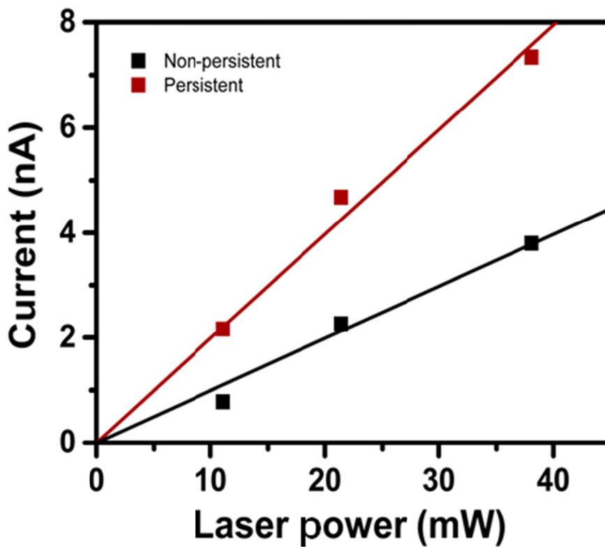
**Figure S10.** Photocurrent versus laser power of TMPyP:TSPP rods illuminated with 445 nm laser light.
