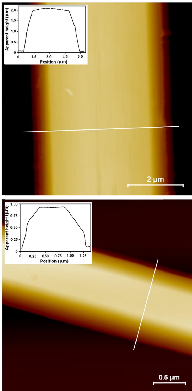
**Figure S4.** AFM images and corresponding cross sectional profiles of two different TMPyP:TSPP crystalline rods.
