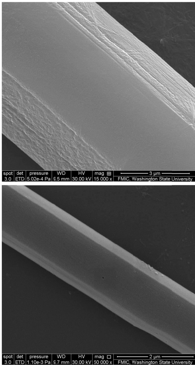
**Figure S5.** SEM micrographs illustrating morphology of a TMPyP:TSPP crystalline rod. The top surface and sloping sides of the crystals are flat with the top face being smoother than the sides.
