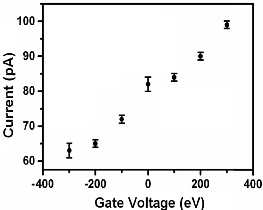
**Figure S8.** Gate Voltage ( $V_G$ ) dependence of the TMPyP:TSPP photoconductivity.  $V_{SD} = 120 \text{ mV}$ . The decrease in current with application of a negative voltage and increase in current with the application of a positive gate voltage is consistent with the behavior of an n-type photoconductor.
