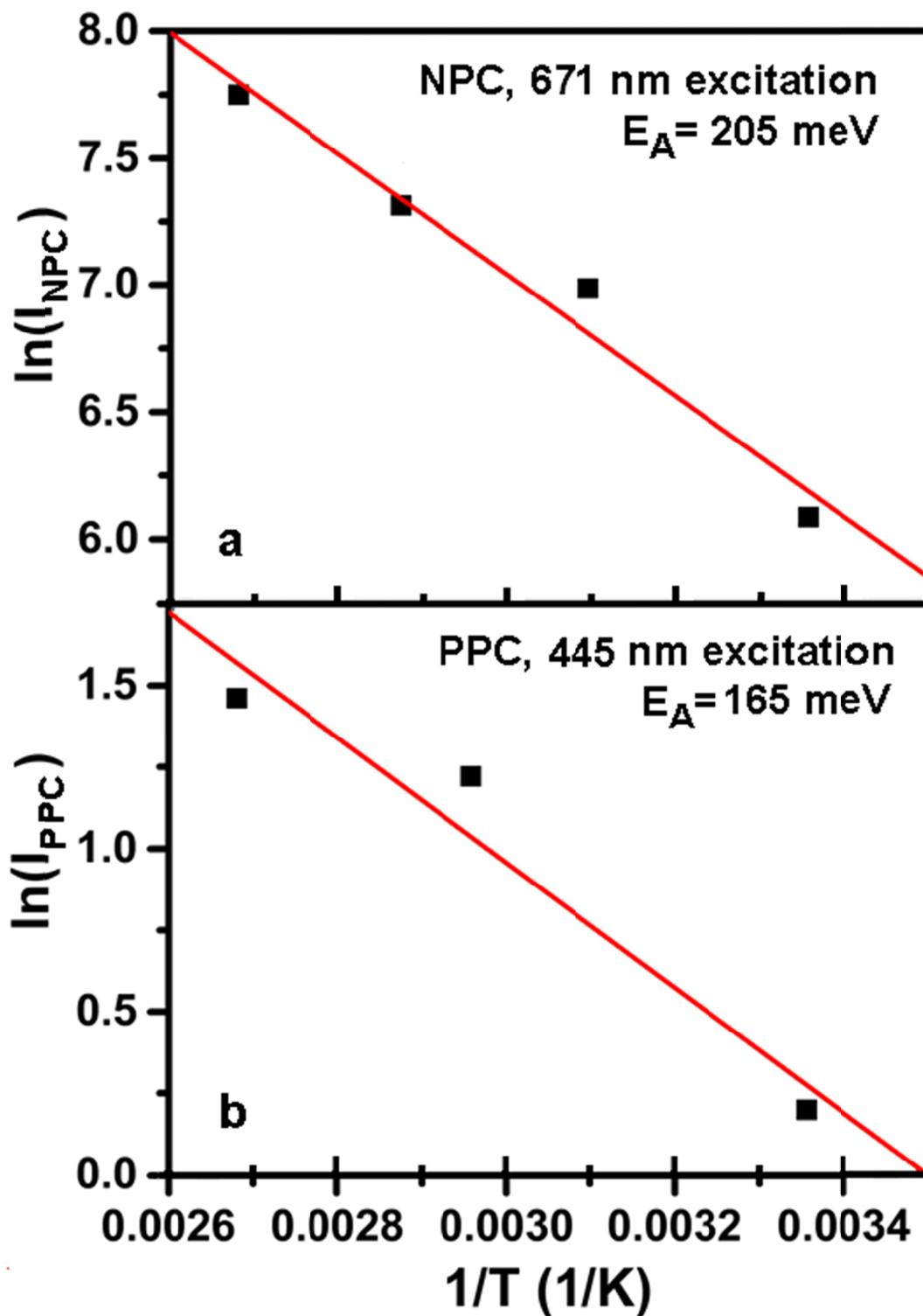
**Figure S12.** Arrhenius plots of the photoconductivity of TMPyP:TSPP assemblies as a function of temperature for: (a) nonpersistent photoconductivity with 671 nm excitation and (b) persistent photoconductivity with 445 nm excitation. Calculated activation energies associated with each plot are shown.
