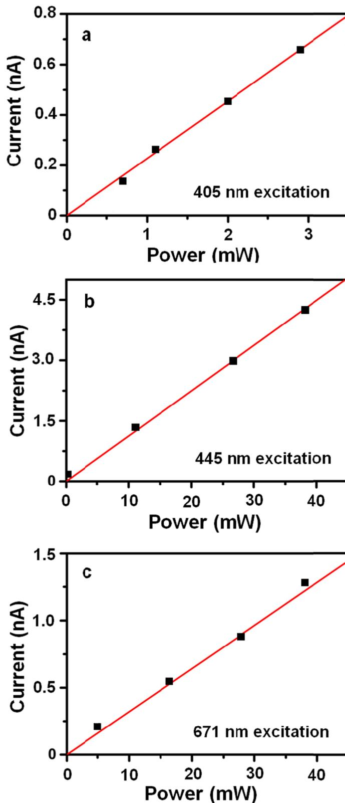
**Figure S7.** Power dependence of the photoconductivity of TMPyP:TSPP measured at different illumination wavelengths. Graph (a) was obtained with 405 nm excitation and has a slope of 0.223 nA/mW. Trace (b) was acquired with 445 nm excitation and has a slope of 0.133 nA/mW. Plot (c) was recorded with 671 nm excitation and has a slope of 0.032 nA/mW.
