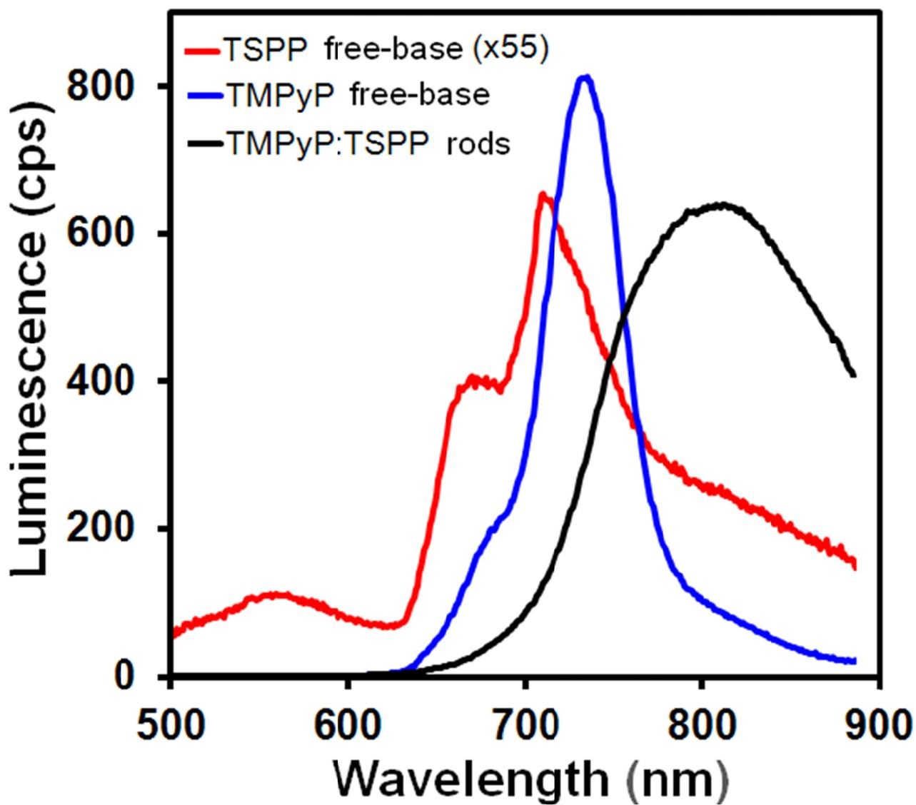
**Figure S9.** Solid state luminescence spectra of free-base forms of the TMPyP and TSPP tectons and the TMPyP:TSPP rods. Note the scale factor on the TSPP emission.
