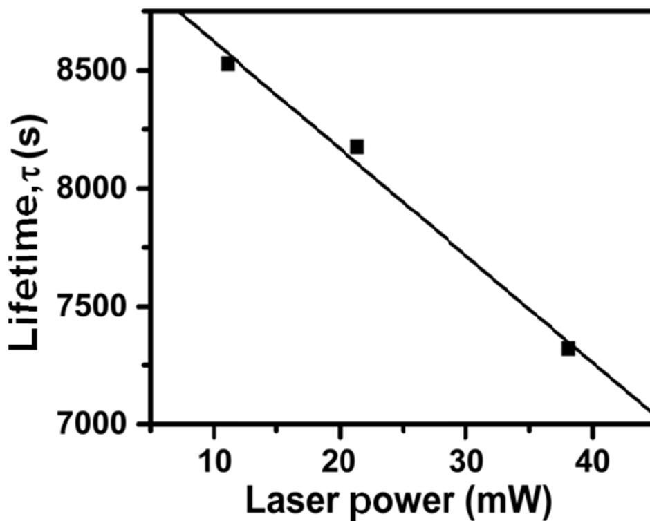
**Figure S11.** Lifetime of PPC versus laser power of TMPyP:TSPP rods illuminated with 445 nm laser light.
