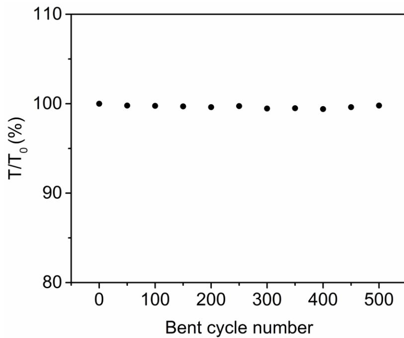
**Fig. S9** Dependence of saturated temperature on bent cycle. Here  $T_0$  and  $T$  correspond to the saturated temperatures before and after bending, respectively.
