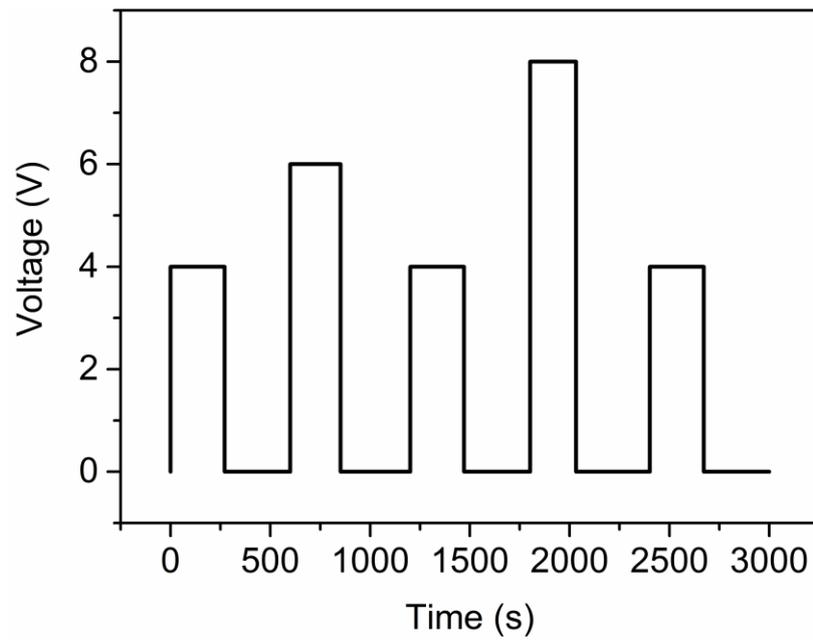
**Fig. S7** Voltage-time curve applied on the strip-shaped TRH.
