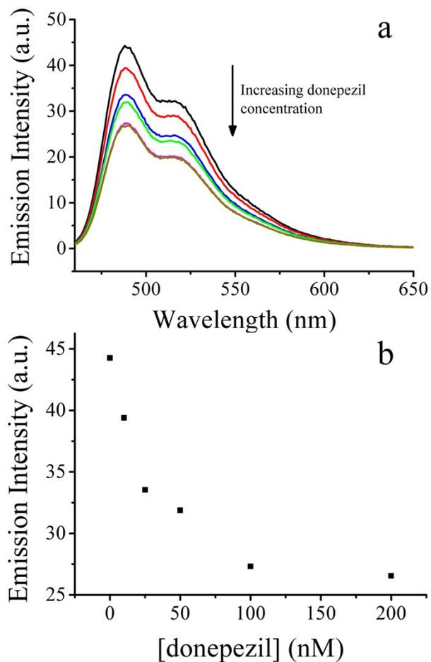
**Figure S14.** Changes in emission spectrum (a) and the corresponding emission intensity at 488 nm (b) of **P-4C+** upon the addition of increasing concentrations of donepezil (0 – 200 nM). Conditions: 5 mM phosphate buffer (pH 7.4), 26.25  $\mu\text{g}/\text{mL}$   $\text{MnO}_2$  nanosheets, 0.3 mM ACh, 50  $\mu\text{M}$  PPi and 100 mU/mL AChE.
