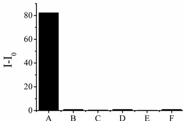
**Figure S9.** Selectivity study. Columns A–G: AChE, lysozyme, ALP, S1 nuclease, trypsin and Exo I nuclease. AChE: 500 mU/mL; the other enzymes: 10 U/mL each. 50  $\mu\text{M}$  EDTA was used instead of pyrophosphate.  $I$  and  $I_0$  represent the emission intensity of  $\text{P-4C}^+$  in the presence and absence of the enzyme.
