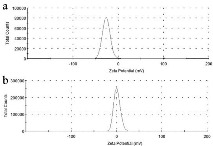
**Figure S3.** Zeta potential analysis: the MnO<sub>2</sub> nanosheets possess a potential value of  $-26.2$  mV before (a) and  $1.29$  mV after (b) mixed with **P-4C+**.
