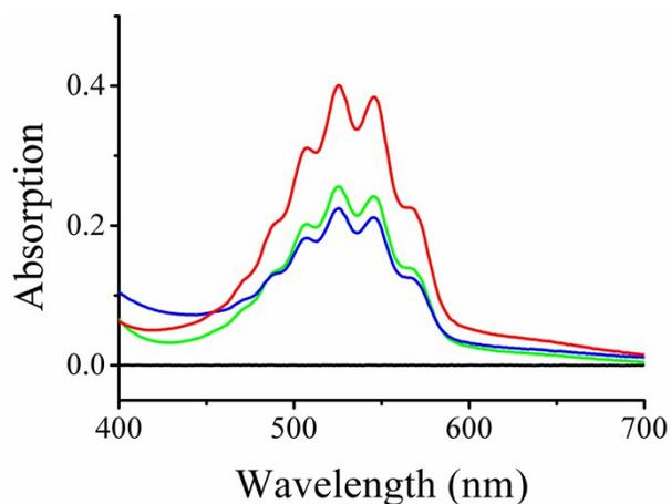
**Figure S6.** UV-vis absorption spectra: Blue curve: the reaction mixture of MnO<sub>2</sub> nanosheets and thiocholine was centrifuged, the supernatant was taken and treated with sodium periodate; Green curve: the reaction mixture of sodium periodate and MnCl<sub>2</sub>; Red curve: KMnO<sub>4</sub> aqueous solution; Black curve (blank control): the MnO<sub>2</sub> nanosheets containing sample solution was centrifuged, the supernatant was taken and mixed with sodium periodate.
