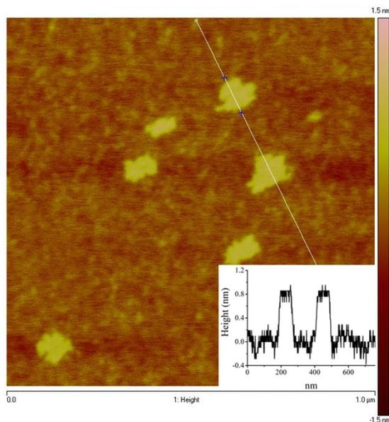
**Figure S1.** Tapping-mode of the AFM image of the MnO<sub>2</sub> nanosheets. Inset: the height profile of the section labeled with the white line.
