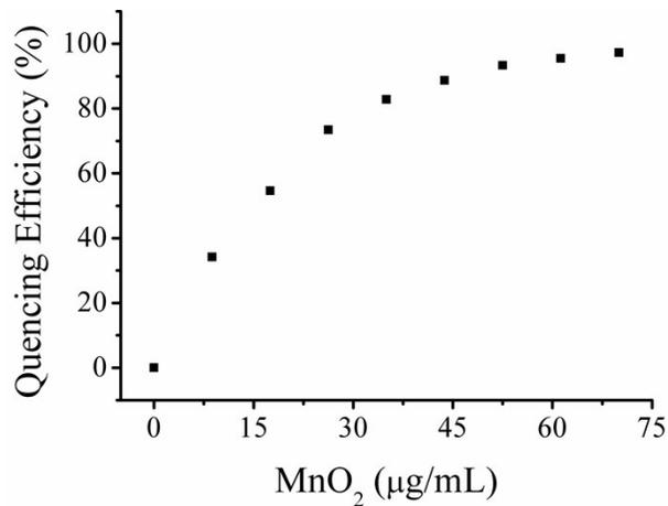
**Figure S4.** Fluorescence quenching efficiency versus MnO<sub>2</sub> nanosheets concentration (0, 8.75, 17.5, 26.25, 35, 43.75, 52.5, 61.25, and 70 µg/mL). Buffer: 5 mM phosphate buffer, pH 7.4.
