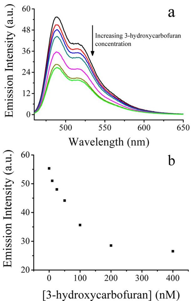
**Figure S15.** Changes in emission spectrum (a) and the corresponding emission intensity at 488 nm (b) of P-4C+ upon the addition of increasing concentrations of 3-hydroxycarbofuran (0 – 400 nM). Conditions: 5 mM phosphate buffer (pH 7.4), 26.25  $\mu\text{g}/\text{mL}$   $\text{MnO}_2$  nanosheets, 0.3 mM ATCh, 50  $\mu\text{M}$  PPI and 100 mU/mL AChE.
