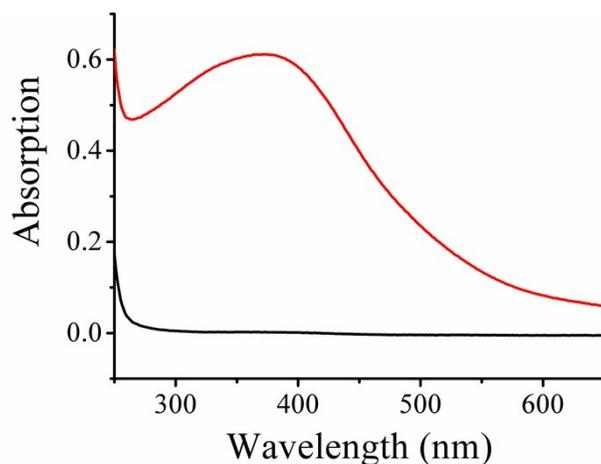
**Figure S7.** UV-vis absorption spectra of the  $\text{MnO}_2$  nanosheets before (red curve) and after (black curve) the enzymatic reaction of AChE with the substrate.
