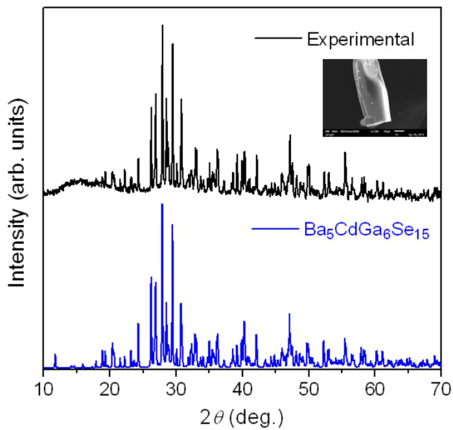
**Figure S1.** Powder XRD pattern of Ba<sub>5</sub>CdGa<sub>6</sub>Se<sub>15</sub>. The inset shows an SEM image of a typical crystal of this compound.
