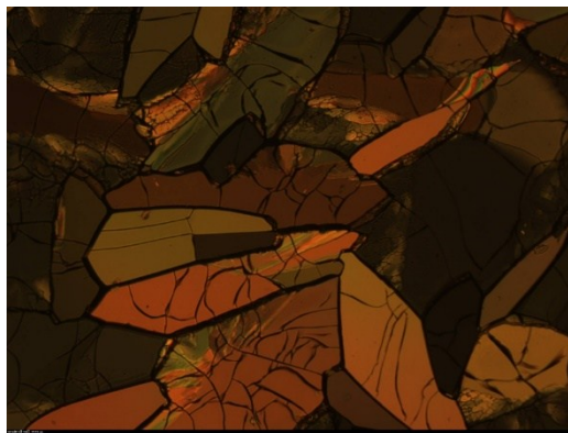
Fig.S59 Mosaic texture observed by POM with of compound T 3,4 D 8 sandwiched between clean glass slides on cooling from isotropic phase at 30°C(left); DSC trace of compound T 3,4 D 8 run at 10°Cmin -1 under N 2 (right).
