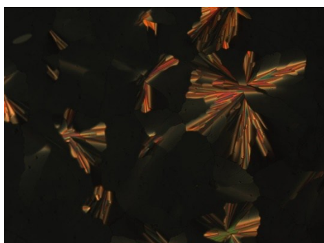
Fig.S71 Fan-shaped texture observed by POM of compound T_{3,5}D_6 sandwiched between clean glass slides on cooling from isotropic phase at 40^{\circ}C (left); DSC trace of compound T_{3,5}D_6 run at 10^{\circ}Cmin^{-1} under N_2 (right).
