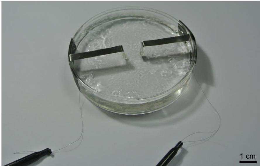
**Fig. S5** Photograph of measuring the ionic conductivity of hydrogel film.
