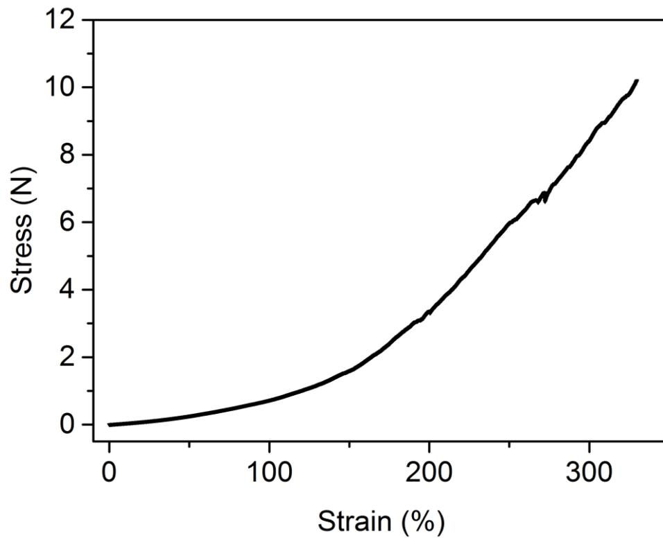
**Fig. S2** Stress-strain curve of the conducting fabric (width of 4 mm and length of 13 mm).
