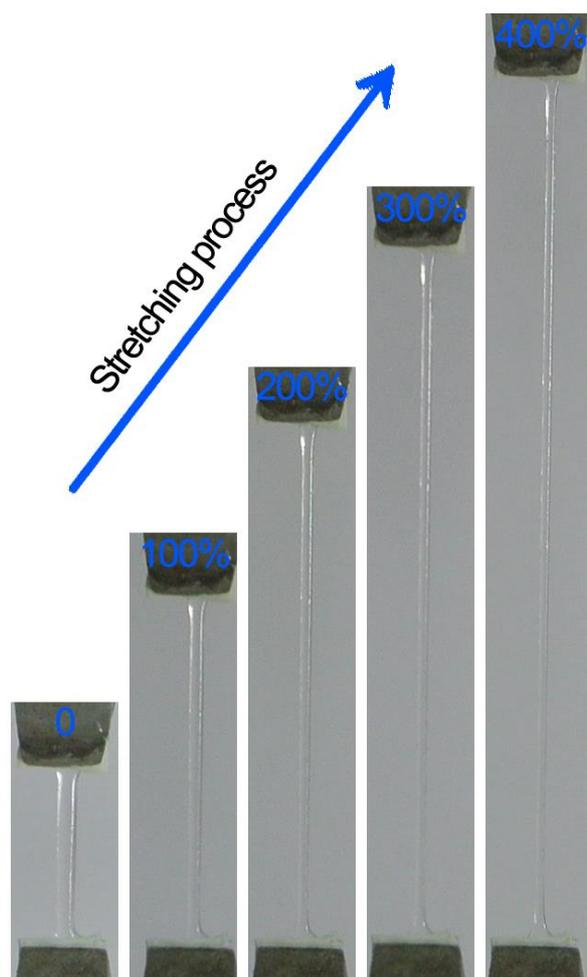
**Fig. S4** Photographs of the hydrogel layer with the increasing strains from 0 to 400%.
