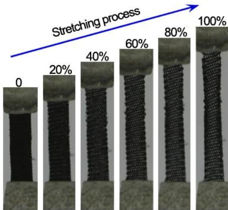
**Fig. S3** Photographs of the conducting fabric at increasing strains from left to right.
