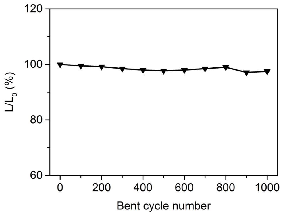
**Fig. S7** Dependence of luminance of the light-emitting fabric on bent cycle number.  $L_0$  and  $L$  correspond to the luminance intensities before and after bending, respectively.
