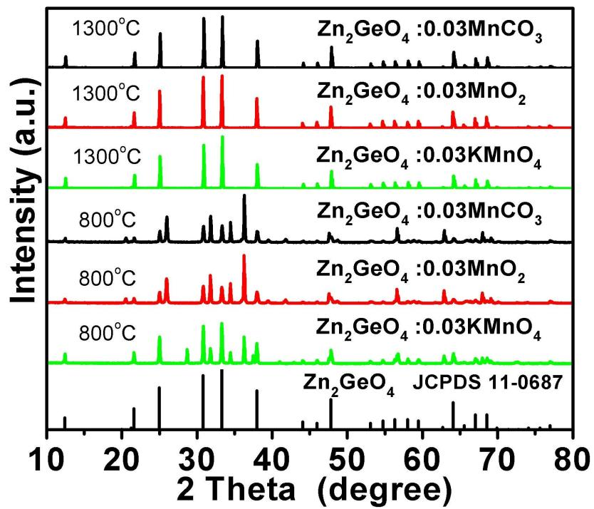
**Fig. S1** The standard XRD pattern of  $\text{Zn}_2\text{GeO}_4$  and measured XRD patterns of  $\text{Zn}_2\text{GeO}_4:0.03\text{Mn}^{2+}$  phosphor with different Mn-sources ( $\text{MnCO}_3$ ,  $\text{MnO}_2$  and  $\text{KMnO}_4$ ) prepared at 1300 and 800 °C, respectively, for 6 h in air condition.
