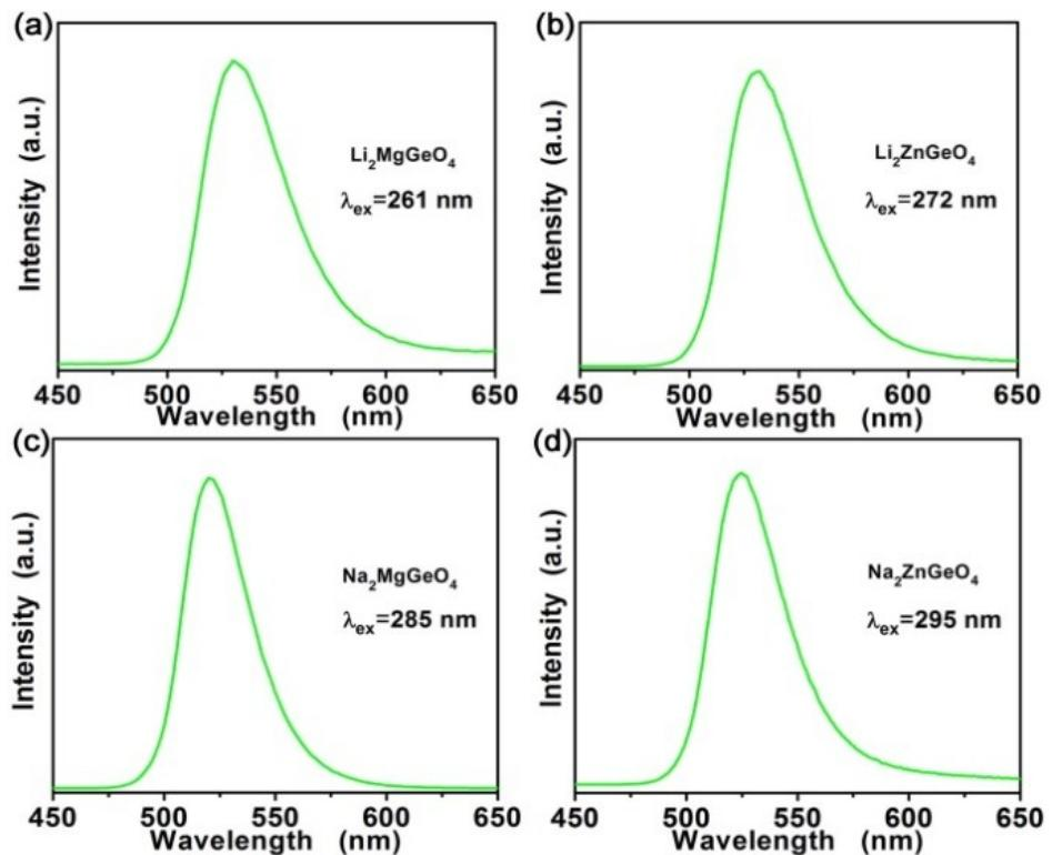
**Fig. S4** PL spectra of (a)  $\text{Li}_2\text{ZnGeO}_4:\text{Mn}^{2+}$ , (b)  $\text{Li}_2\text{MgGeO}_4:\text{Mn}^{2+}$ , (c)  $\text{Na}_2\text{MgGeO}_4:\text{Mn}^{2+}$ , and (d)  $\text{Na}_2\text{ZnGeO}_4:\text{Mn}^{2+}$  phosphors prepared by using  $\text{KMnO}_4$  as Mn source.
