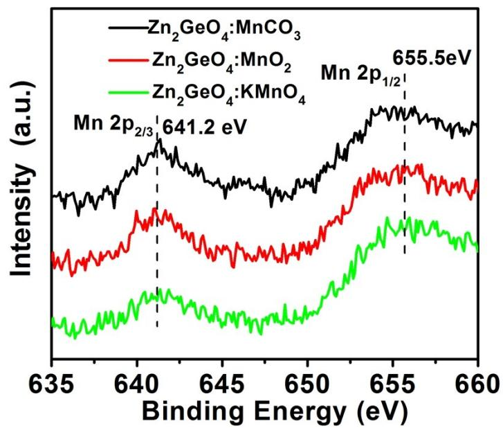
**Fig. S2** XPS spectra for Mn 2p region in  $\text{Zn}_2\text{GeO}_4:\text{Mn}$  samples synthesized by using different Mn-sources ( $\text{MnCO}_3$ ,  $\text{MnO}_2$  and  $\text{KMnO}_4$ ).
