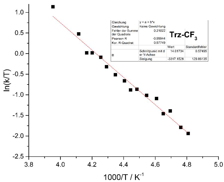
Figure S21. Eyring plot of  $\text{Trz-CF}_3$ .
