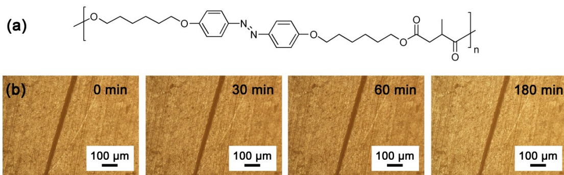
Fig. S2 (a) Chemical structure of poly(4,4'-bis(6-hydroxyhexyloxy)azobenzene methylsuccinate) (PBHMS). (b) Unsuccessful self-healing process of PBHMS at 60 °C under the POM. After isothermal process at 60 °C for 180 min, the scratched film remained un-healed.
