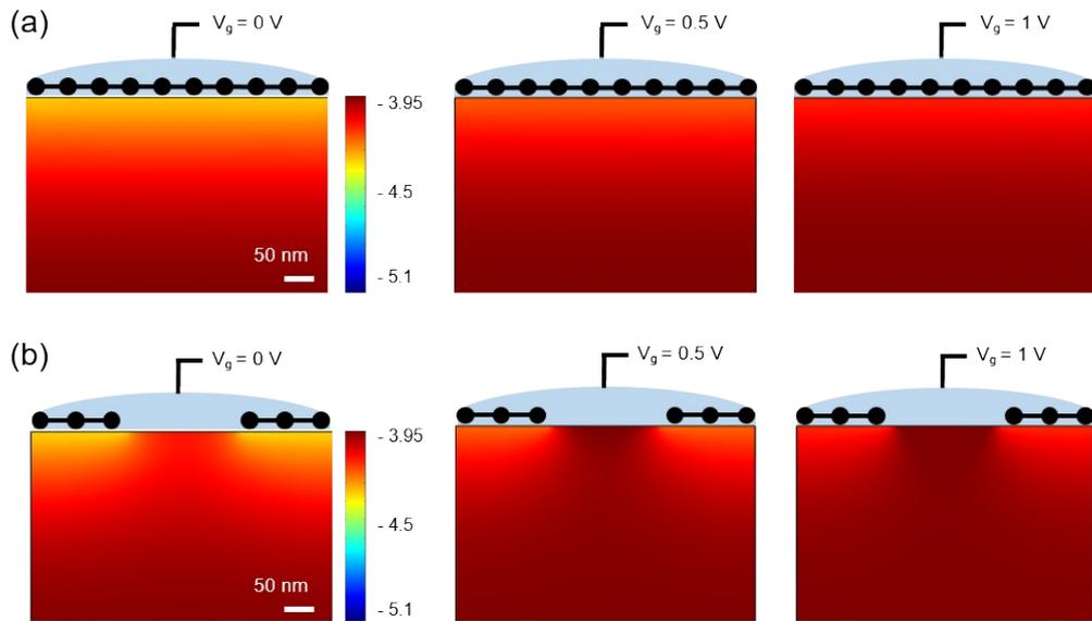
**Figure S2.** FEA simulation results for Gr-Si (a) and GM-Si (b) SJSCs with positive  $V_g$ .
