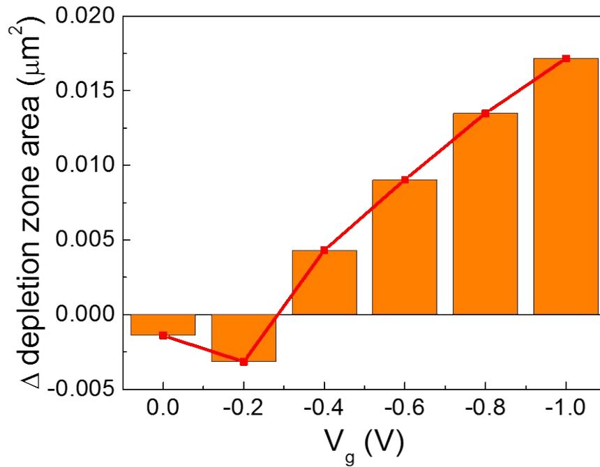
**Figure S1.** The difference of depletion zone areas between Gr-Si and GM-Si Schottky junctions (i.e., depletion area of GM-Si Schottky junction – depletion area of GM-Si Schottky junction) in Figure 4. The depletion zone was defined as the region whose electrical potential is smaller than 4.26 eV (dotted lines in Figure 4).
