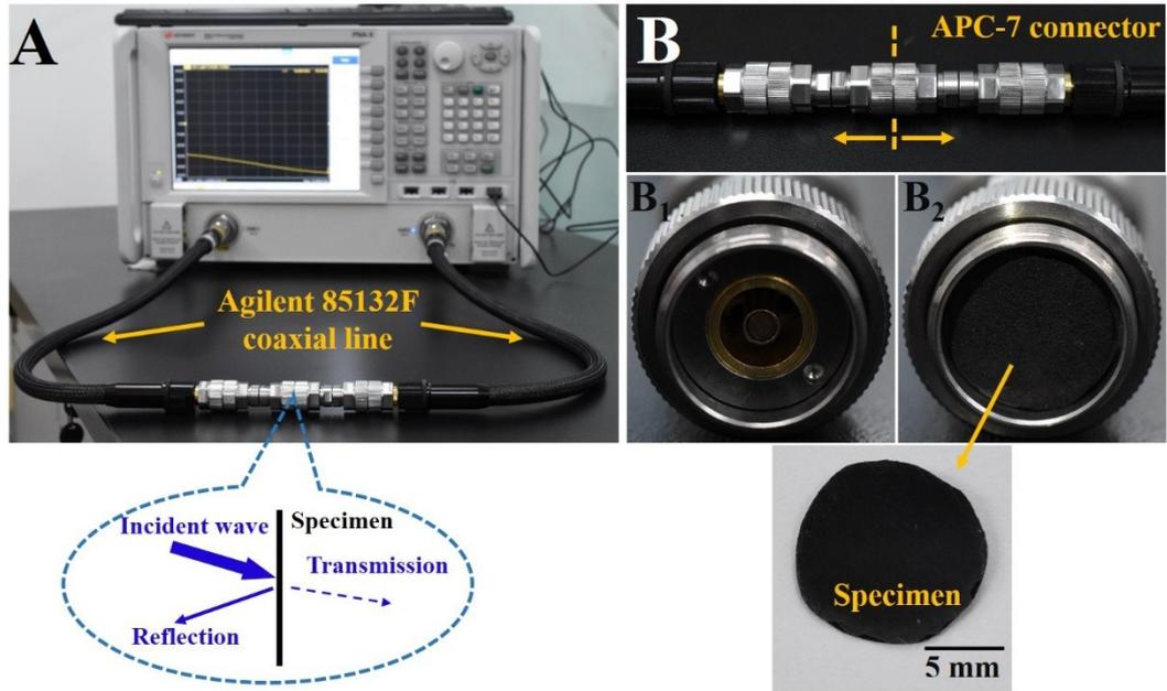
2 Fig. S1 EMI shielding measurement setup and specimen.
