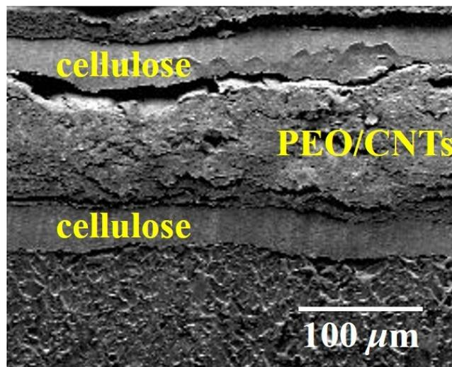
4 Fig. S2 SEM image of layer-structured CNTs/cellulose film.
