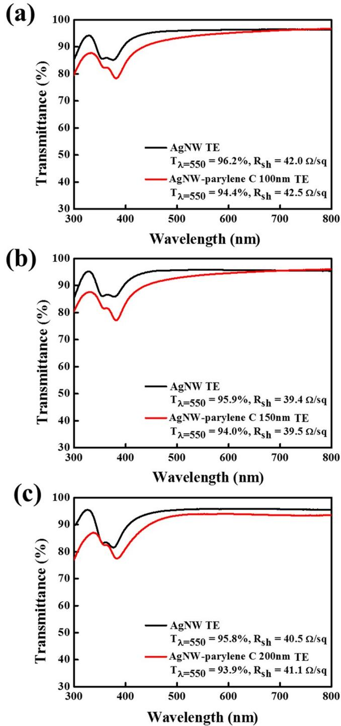
**Fig. S2** Optical transmittance spectra and sheet resistances of AgNW-parylene C TEs with various thickness of parylene C layers (a) 100nm, (b) 150nm, (c) 200nm.
