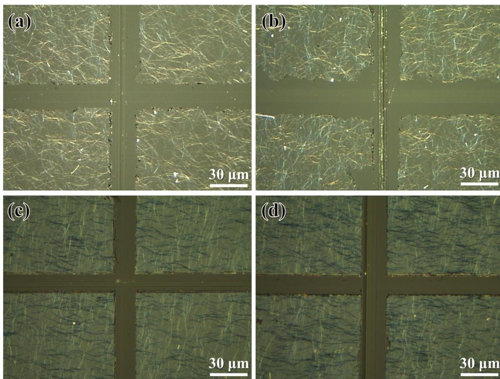
**Fig. S6** OM images of (a), (b) AgNW and (c), (d) AgNW –parylene C TEs which have the square lattice patterns before and after cross-cut test with a 3M scotch tape.
