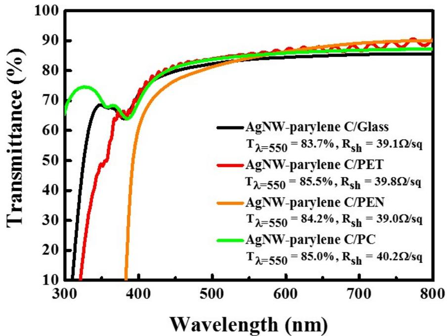
**Fig. S7** Optical transmittance spectra and sheet resistance values of AgNW-parylene C TEs prepared onto various substrates such as glass, PET, PEN, and PC.
