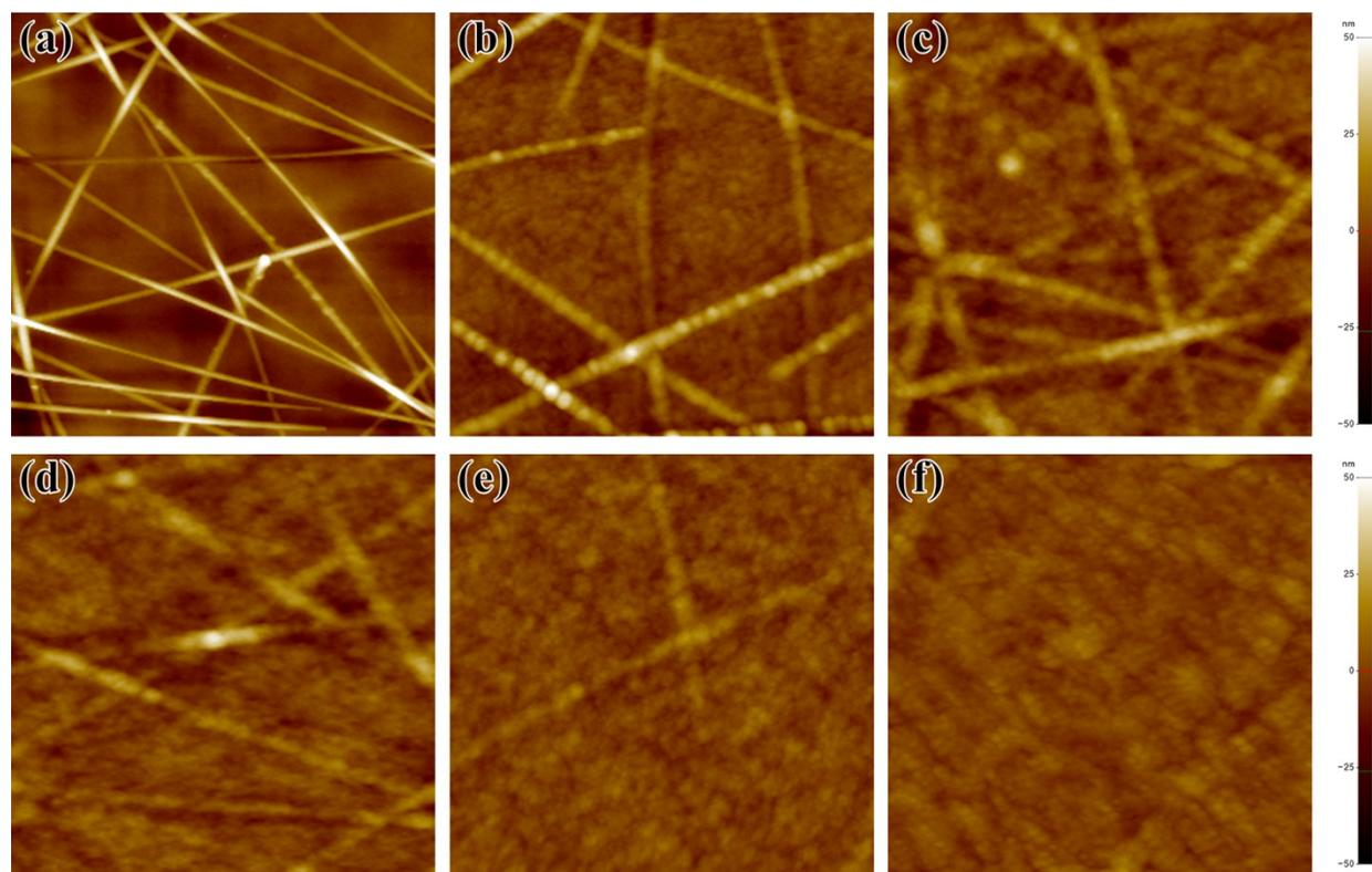
**Fig. S4** AFM topographies of (a) AgNW and AgNW-parylene C TEs with various thickness of parylene C protection layers (b) 25nm, (c) 50nm, (d) 100nm, (e) 150nm, and (f) 200nm.
