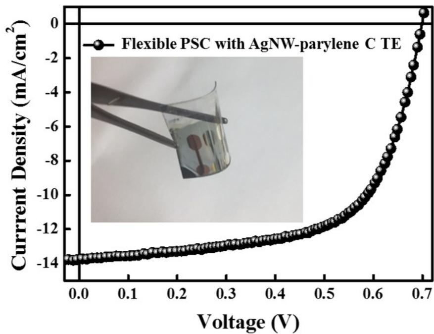
**Fig. S11** Current density–voltage ( $J$ – $V$ ) characteristics of flexible bulk heterojunction (BHJ) polymer solar cell with AgNW-parylene C/PET TE. The inset shows the photograph of the flexible BHJ PSC with AgNW-parylene C/PET TE.
