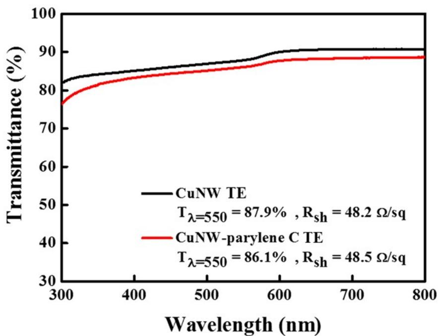
**Fig. S9** Optical transmittance spectra and sheet resistance values of CuNW and CuNW-parylene C TEs.
