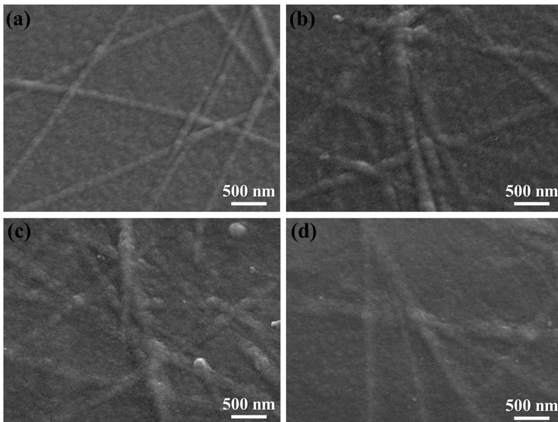
**Fig. S8** SEM images of (a) AgNW-parylene C 50nm, (b) AgNW-parylene C 100nm, (c) AgNW-parylene C 150nm, and (d) AgNW-parylene C 200nm TEs after the long-term stability test at 70 °C and 70% RH.
