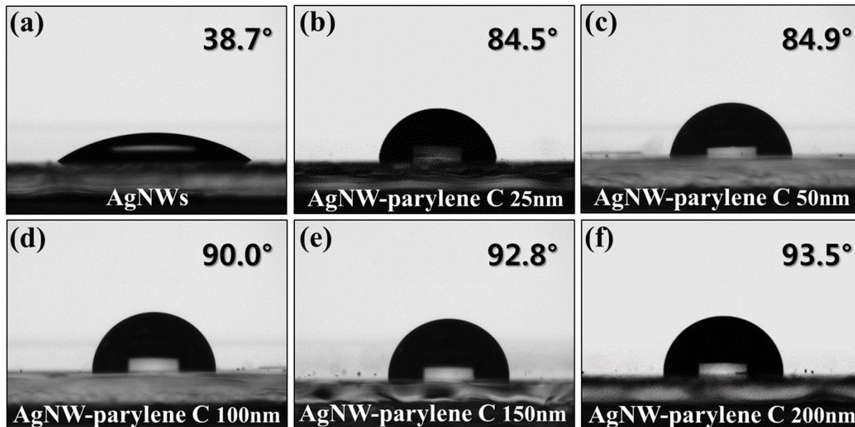
**Fig. S1** Contact angle measurements of (a) the AgNW and AgNW-parylene C TEAs with (b) 25nm, (c) 50nm, (d) 100nm, (e) 150nm, (f) 200nm parylene C layers using deionized water droplet.
