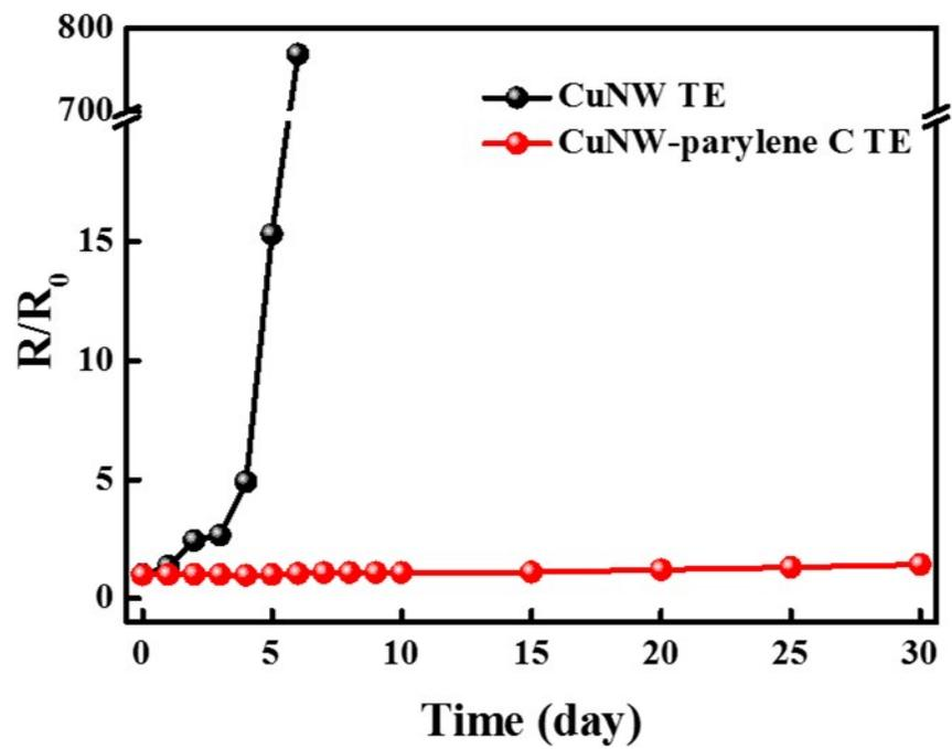
**Fig. S10** Sheet resistance change of CuNW and CuNW-parylene C TEs during the long-term stability test at ambient condition for 30 days.
