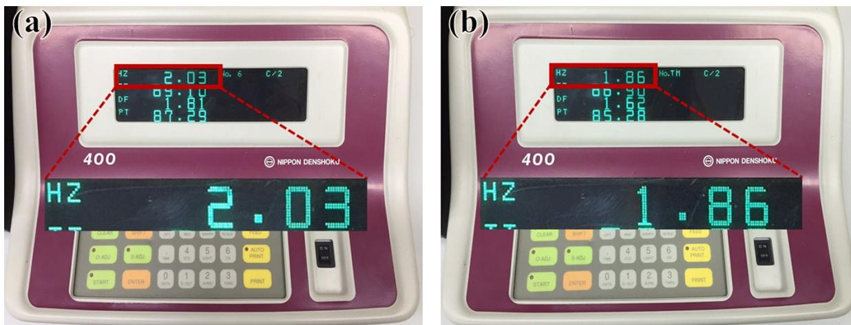
**Fig. S5** Haze test of (a) AgNW/PET and (b) AgNW-Parylene C/PET TEs.
