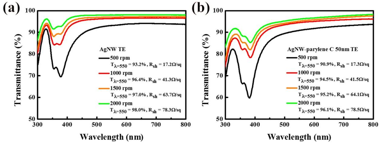
**Fig. S3** Optical transmittance spectra and sheet resistances of AgNW and AgNW-parylene C TEs with the spin coating speed from 500 rpm to 2000 rpm.
