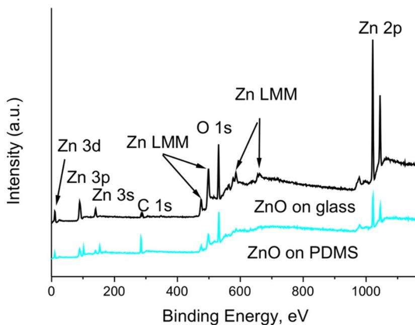
**Fig. S1** X-ray photoelectron spectroscopy (XPS) survey of the ZnO-Nrd coated substrates: glass vs PDMS. The peaks show the presence of Zinc for as-prepared NRs as well as signals due to the Auger transitions.
