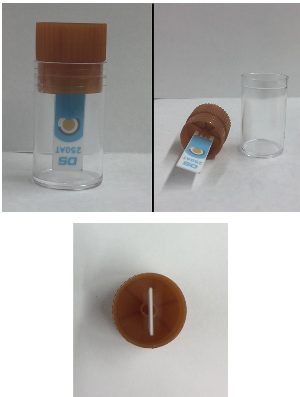
Figure S1. Transport device of the SPGE to the laboratory, based on a plastic vial with a fitting cap
